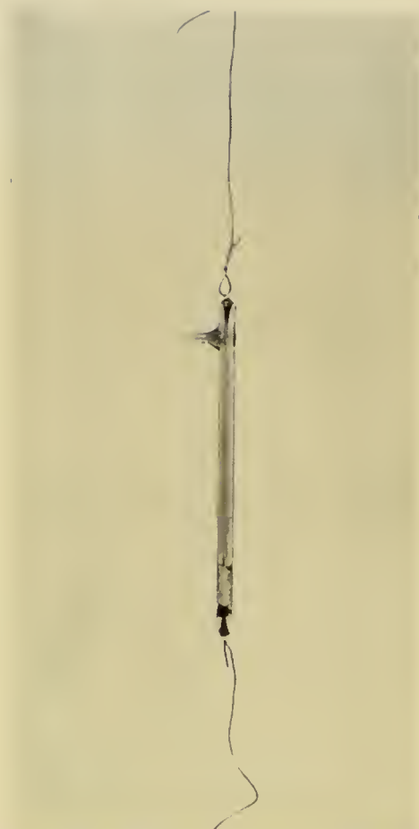
FIG. 21. Original Spectrum-Tube in which the formation of Helium from Radium was first observed.
