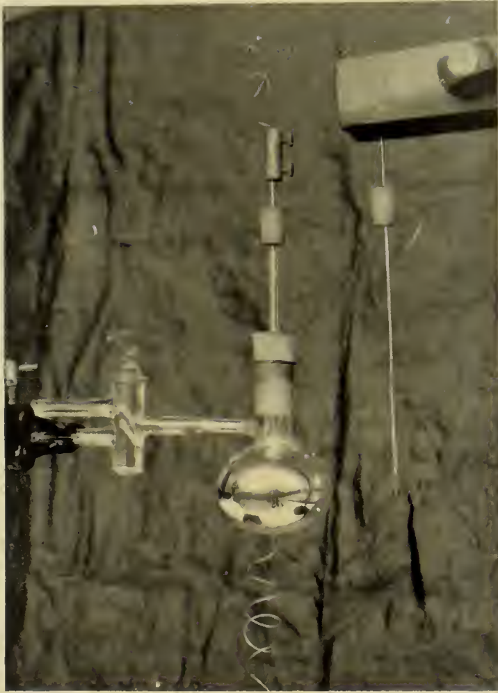
FIG. 29. Apparatus for obtaining the Active Deposit of Radium.
