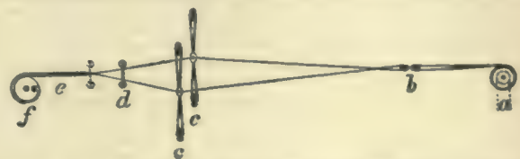
FIG. 26.—Section of Plain Web in Process of Weaving on the Loom. a, The warp beam. d, The reed in position for picking, and also for beating-up. b, The lease rods by which the warp is divided and crossed. e, Woven cloth. c, c, Two pairs of shafts containing healds. f, The cloth beam.
