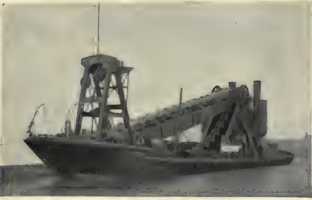
FIG. 3.—Barge-loading dredger, "St Austell," constructed for the British Government by Wm. Simons & Co.
