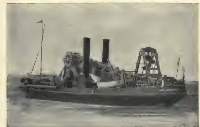
FIG. 8.—Twin-screw hopper-dredger, "Percy Sanderson," built for the European Danube Commission by Wm. Simons & Co.
