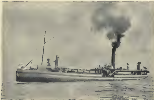
FIG. 7.—Twin-screw sand-pump dredger, "Kate," built for the East London Harbour Board by Wm. Simons & Co.
