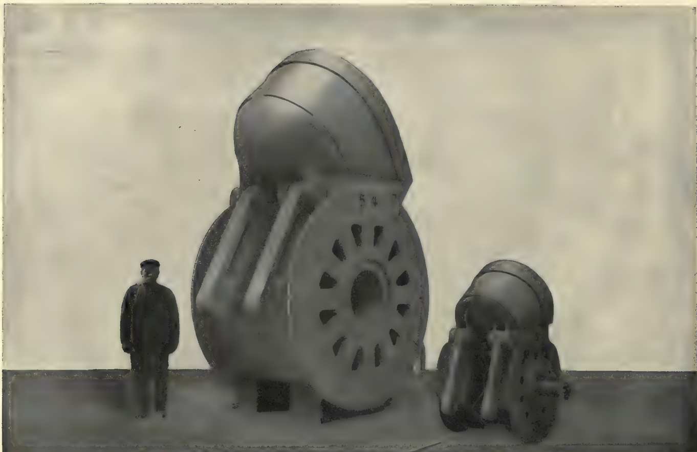
FIG. 11.—BUCKETS OF 5 AND 54 CUBIC FEET CAPACITY COMPARED. The latter, the largest ever made, were for the hopper-dredger "David Dale" (Plate I. fig. 10), built by Lobnitz & Co.
