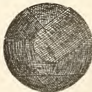
Elastic Fabric Center, Wound Under Tension, with Inside of India-rubber Thread Wound Under Tension. [Patent No. 696,888—E. Kempshall.]
