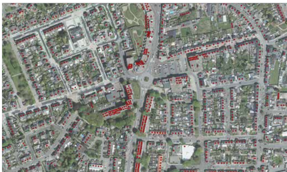
Figure 3. Aerial picture of the City of Heerlen: green dots are roofs with solar panels, red dots without
