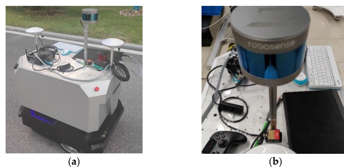
Figure 11. (a) Outdoor autonomous mobile robot experimental platform equipped with GPS, LiDAR, and IMU sensors for data collection; and (b) closer view of the LiDAR and IMU sensors.
