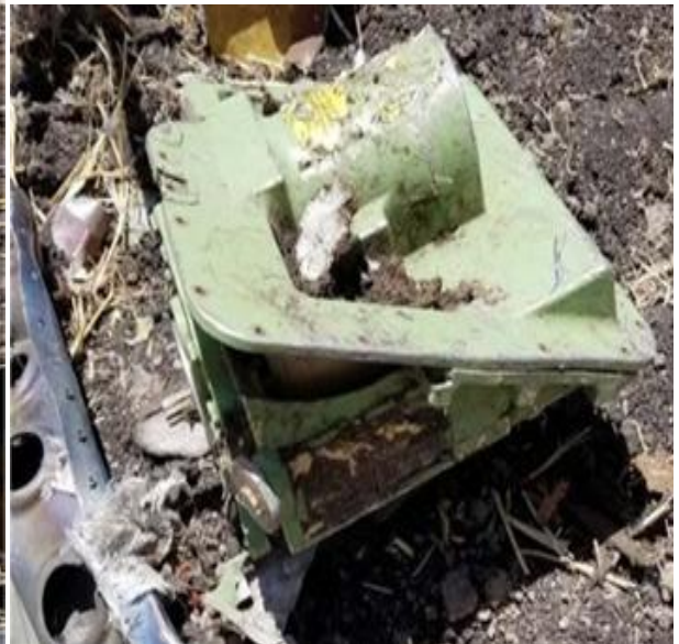
FIGURE60: STAB TRIM ELECTRIC MOTOR HOUSING
