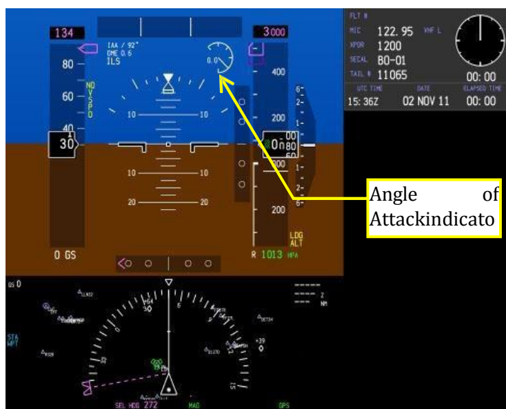
Figure 10: AOA Indicator on PFD
