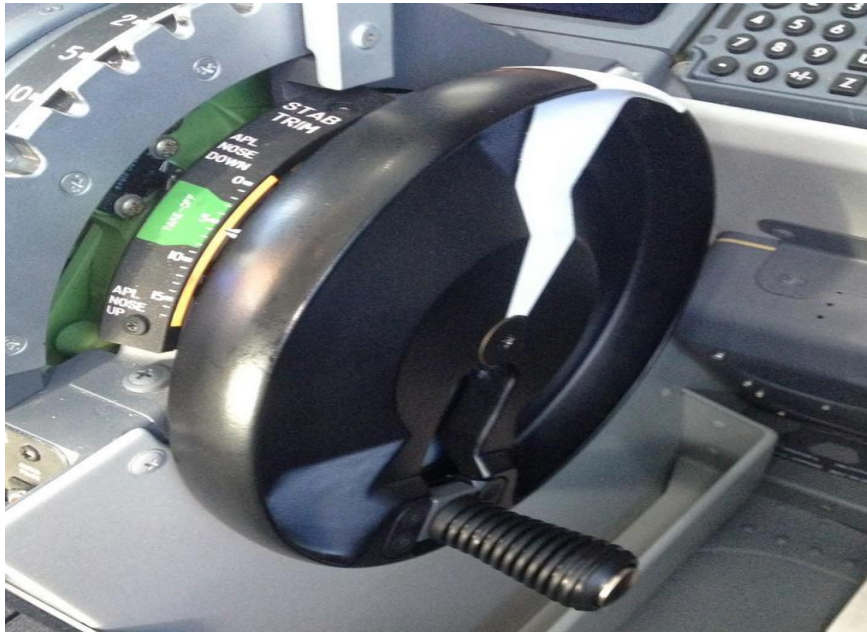
FIGURE 19: THE TRIM WHEEL, WITH THE HANDLE EXTENDED
