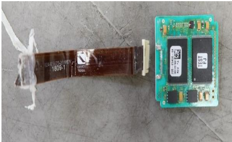
FIGURE 3: FDR MEMORY BOARD, FLEX AND CONNECTOR
