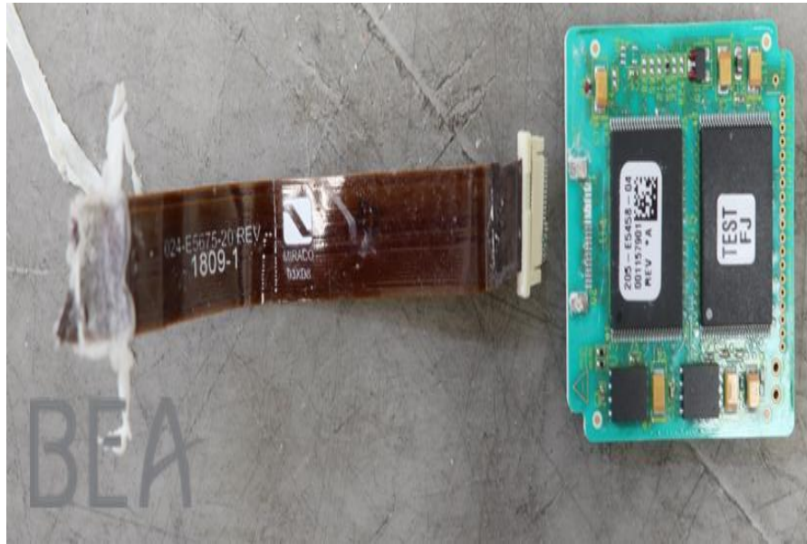
FIGURE 34: FDR MEMORY BOARD, FLEX AND CONNECTOR
