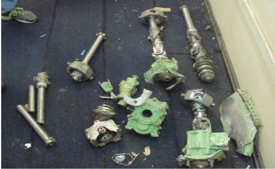
FIGURE56: TRAILING EDGE FLAP TRANSMISSIONS AND BALL SCREWS
