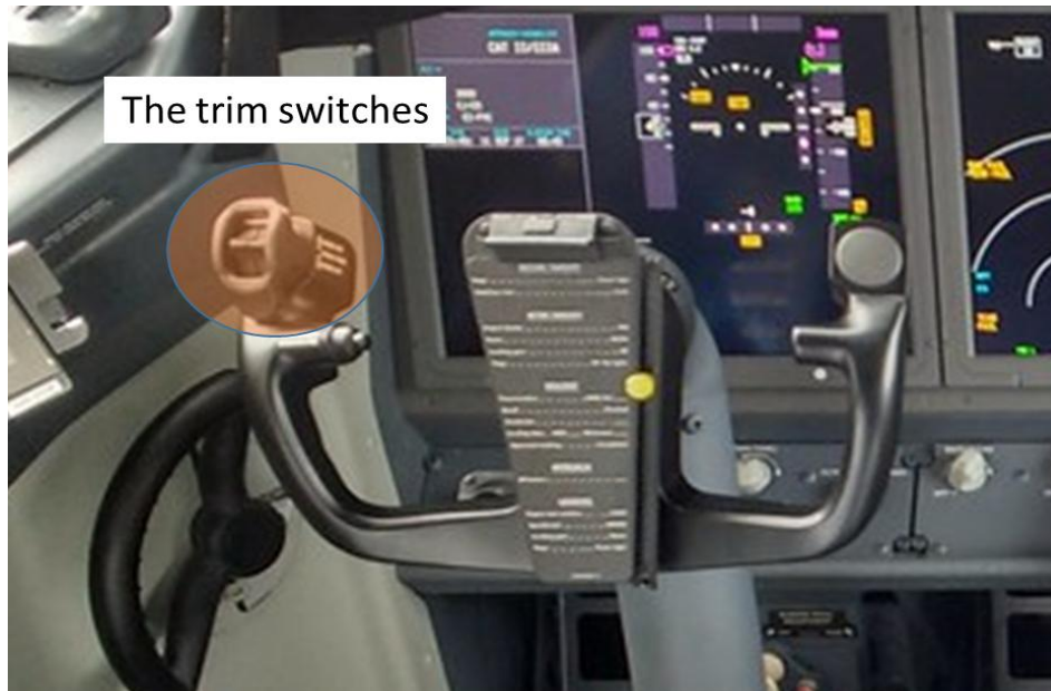
FIGURE 18: TRIM SWITCHES ON THE LH YOKE
