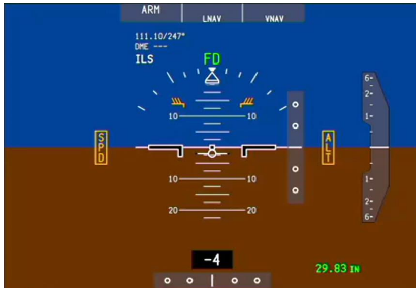
Figure 5: Instrument SPD and ALT flags appear on PFD
