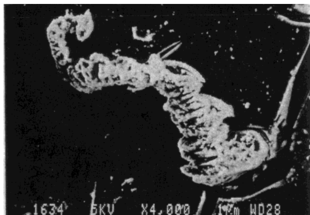
Figure 3. Micrograph of a single dendrite lithium grown in PC. (Reproduced with permission from ref 57 (Figure 6a). Copyright 1989 The Electrochemical Society.)
