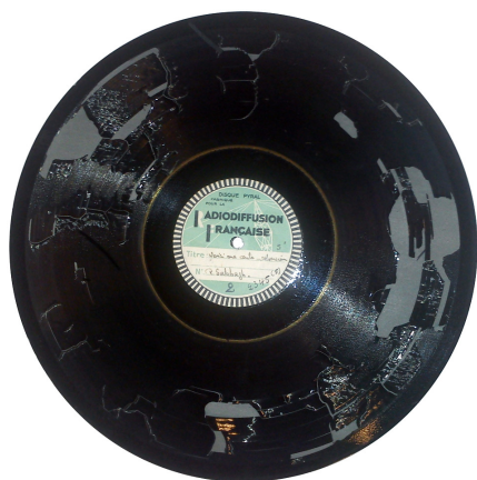
Figure 5: A zinc-based de-laminating lacquer disc record with lacquer curling and missing patches
