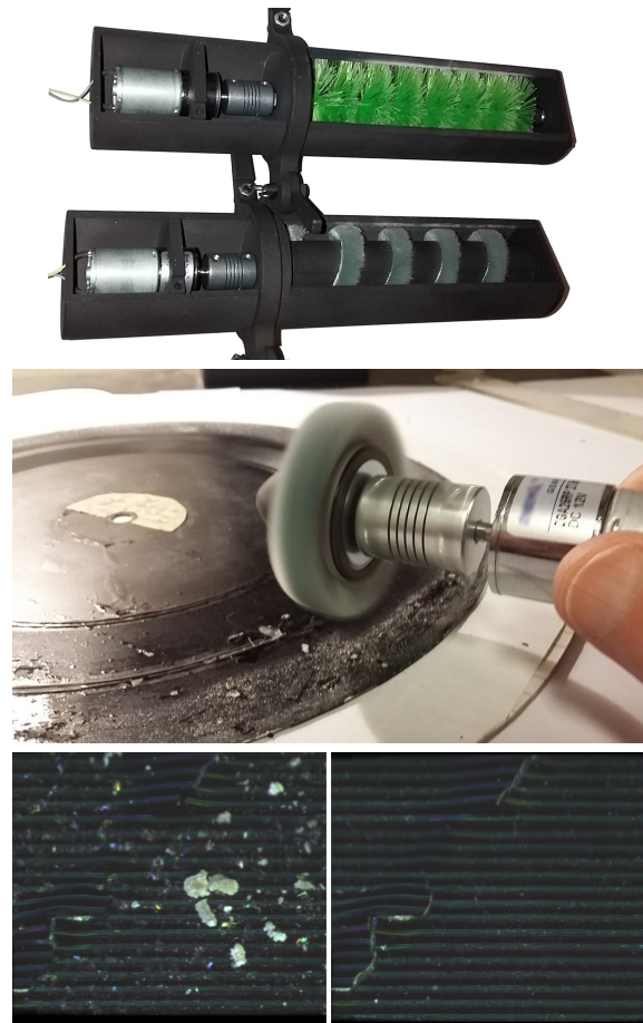
Figure 8: Top: stiff and soft roller brushes usable for robust cracked records. Center: using a hand-held soft rotary brush to eliminate exudates and dust from fragile discs. Bottom: the same 8x6mm area from same disc before and after brushing.
