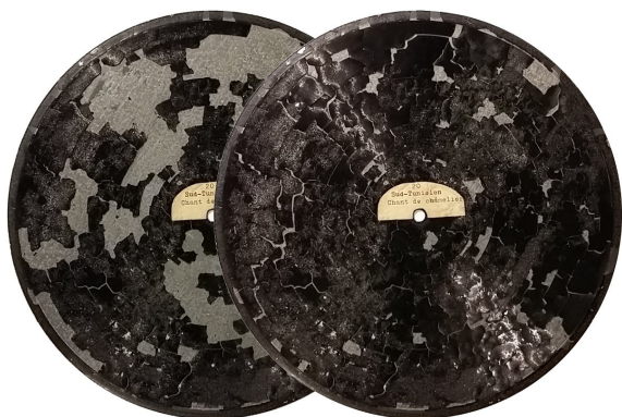
Figure 9: One zinc-based record, before and after brushing and replacing missing flakes (playback in progress).
