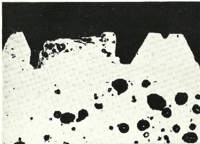
FIG. 16. Section through a slug. The centre character is porous and crumbly Magnification: 25 times
