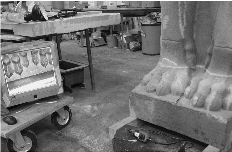
1.2 The feet of one of the human-headed lions from the entrance to the throneroom of Ashurnasirpal II now in the British Museum. The 3-dimensional data was recorded using a NUB 3D Triple White light scanning system and milled at a resolution of 400 microns. On the computer screen is an image of the scanned data which is directly compared to the facsimile to ensure accuracy. Photograph by Factum Arte
