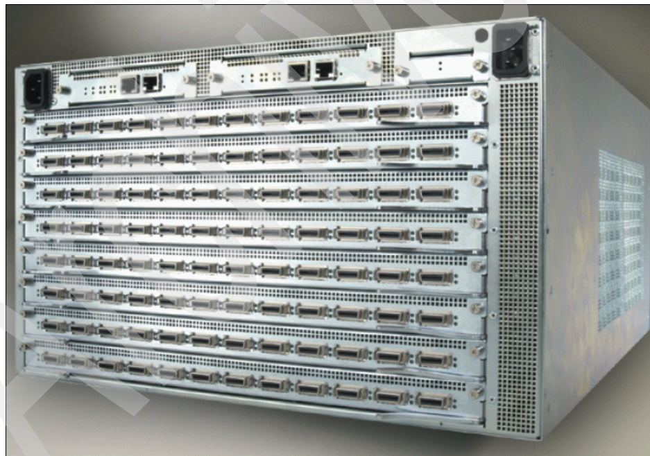
Figure 3-9 Rear view of the SFS 7008P InfiniBand switch
