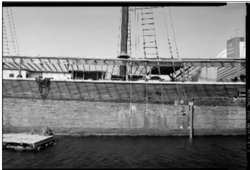
Figure 38. Port hull of Wawona showing the mainmast chainplates. Source: Library of Congress.
