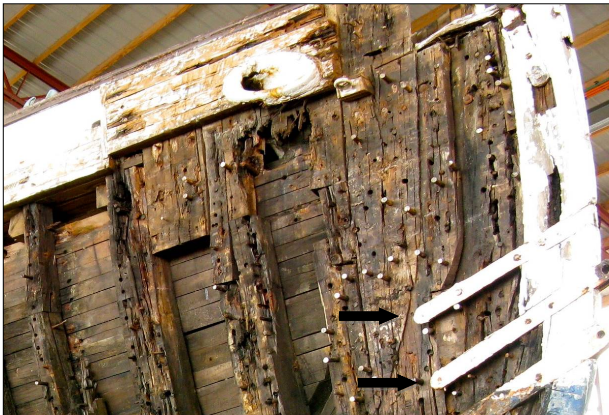
Figure 30. Bow of Coronet (1885) showing the bobstay fasteners on the stem. Source: Daniels 2010.
