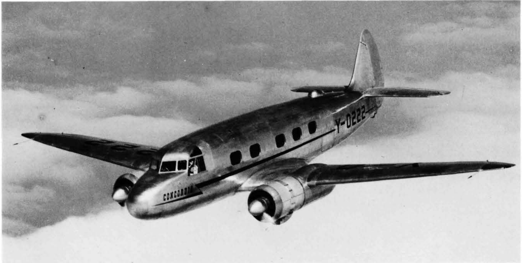
Above: The Cunliffe-Owen Concordia 10-seater Y-0222 was a nice-looking prototype, seen in a photo session soon after its first flight piloted by A. Corbin on 19.5.47. It was powered by two 505 rated hp Alvis Leonides 9-cyl radial engines and had an economical cruise of 190 mph. (via Jack Meaden)
