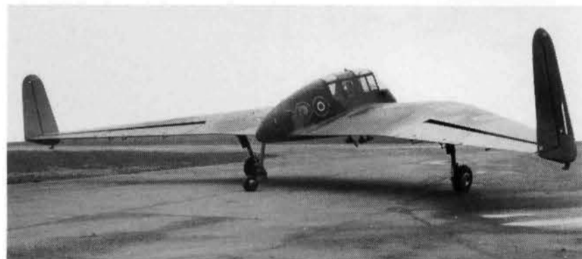
Top: The first GAL.56 TS507, "Medium V" with 28.4° sweepback. Note the Zaunkönig behind.
