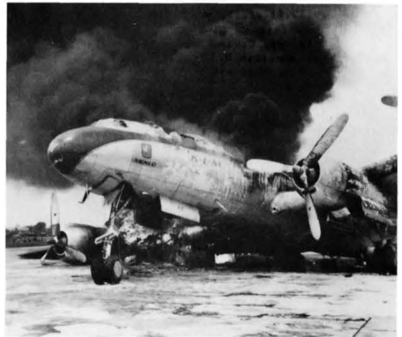
Above and below: KLM Constellation PH-TFF burning at Don Muang, Bangkok on 23.3.52. The missing no.3 engine and collapsed right undercarriage are obvious, the fire crews are not. (via Ronald Dijkstra)
