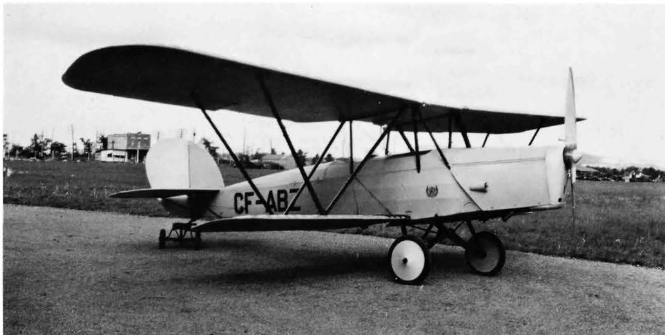
Left: This example of a Curtiss-Reid Rambler III CF-ABZ c/n 1020 was not a club aircraft although many of the type were operated under the DND scheme. It was brought to England by its owner, J.C. Webster of the Montreal Light Aeroplane Club, in 1931 to take part in the Kings Cup Air Race. Powered by a DH Gipsy III, it finished in thirteenth place.
