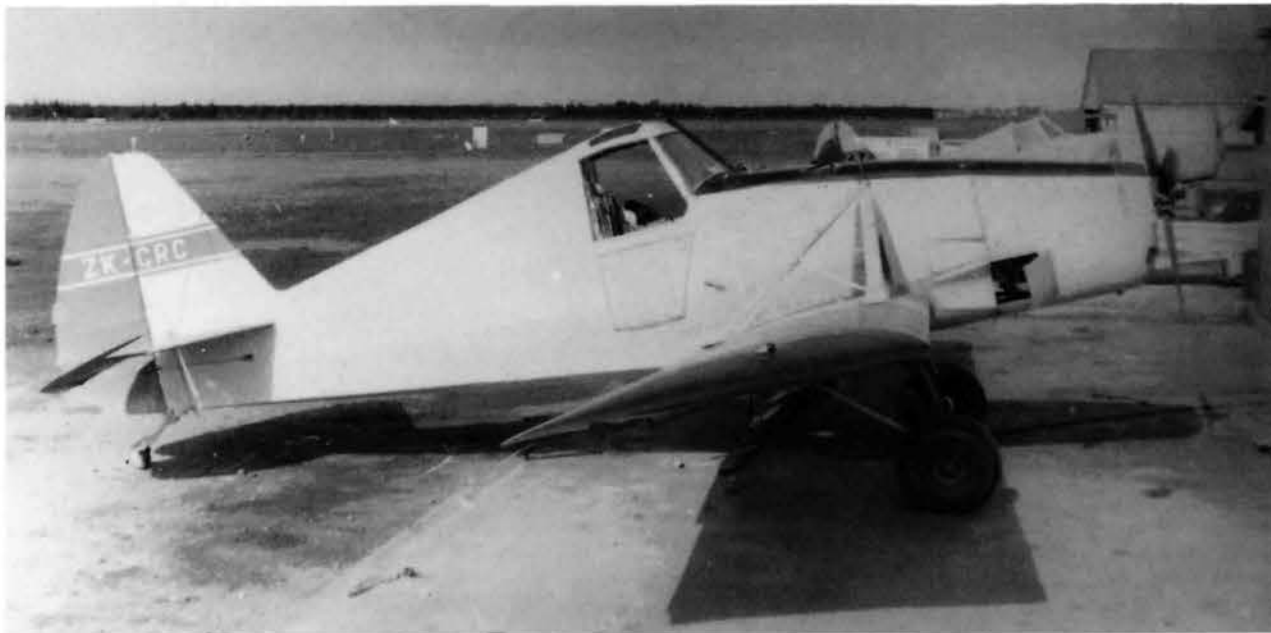
Left: Eight Callair B-1 agricultural aircraft were imported into New Zealand during 1966. ZK-CRC is seen here, with -CRJ behind, possibly when both were used by Auster Air Services in 1973. The Callair was built by Inter Mountain Manufacturing Co of Afton, Wyoming, and was powered by a 400 hp Lycoming IO-720-A1A flat eight, though in 1967 ZK-CRU was converted to a 450hp Pratt & Whitney R-985 nine-cyl radial as a B-1A. (R.W.Kerr)
