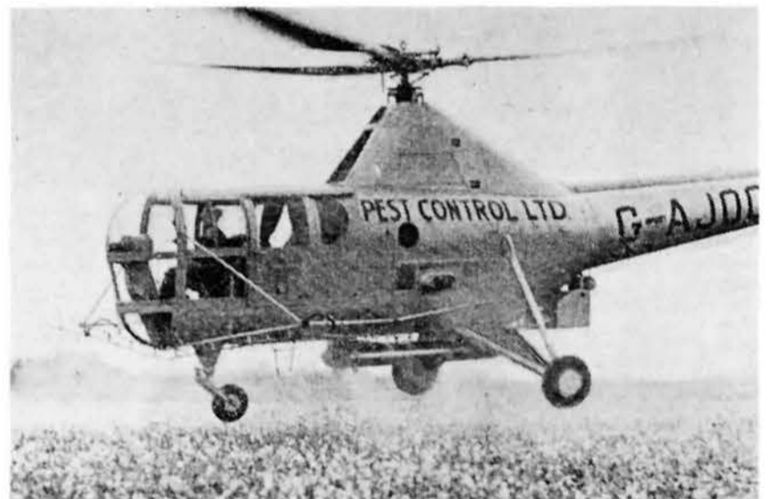
Above: Pest Control's Sikorsky S-51 G-AJOO showing its 65 gallon belly tank, rear-mounted pump unit and short spray booms during a spraying demonstration. See item 17.6.48. (Flight via Jack Meaden)
