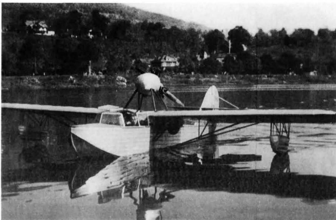
Above: The 1939 Applegate Duck amphibian was dropped by Piper after trials but became the inspiration for the 1944 Goodyear Duck (see "What Do You Know" in "Digest" Spring 1989). It is shown here in 55hp form, registered NX27960. (via Jack Meaden)
