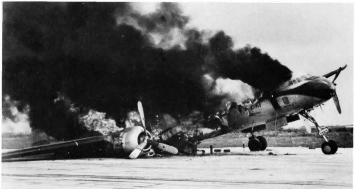
Above and below: KLM Constellation PH-TFF burning at Don Muang, Bangkok on 23.3.52. The missing no.3 engine and collapsed right undercarriage are obvious, the fire crews are not. (via Ronald Dijkstra)
