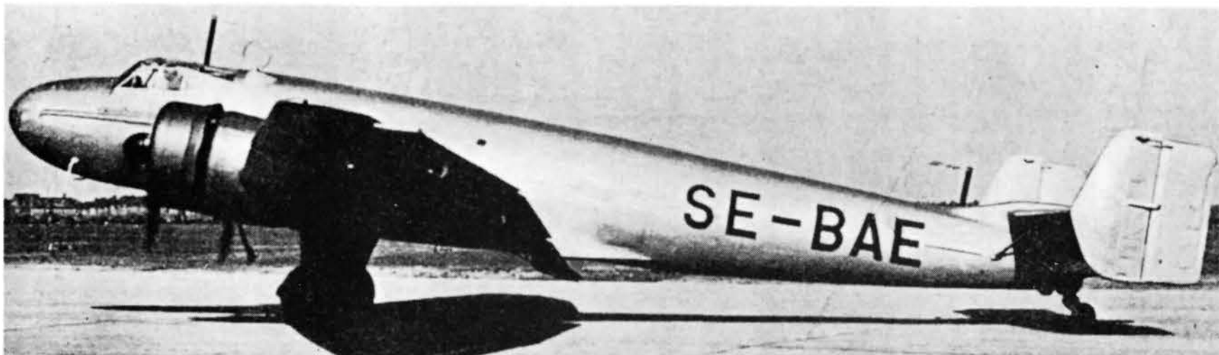
Above: One of the three visiting Swedish Junkers (see Extract 18.6.48) was the Ju 86 Z-7 / Tp9 Fv911. Shown here in 1938 as mail carrier SE-BAE "Svalan" it later had cabin windows added and Mercury engines substituted for Hornets.
