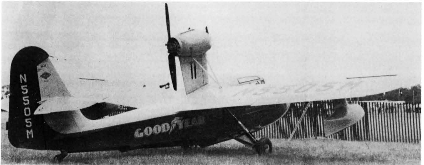
Below: NC5505M shows the trial installation of a second step to the hull to obtain a better unstick on take-off.
