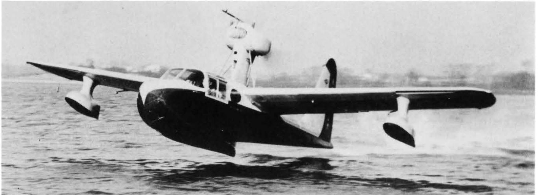
Above: N5512M taking off with the one-step NACA hull fitted and a test pitot mounted on the engine nacelle. (Howard Levy)
