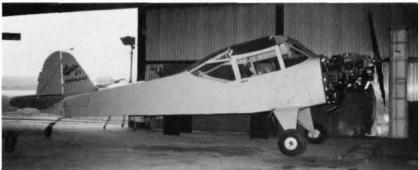
Above: G-AJIT was worked on without wings to keep down hangarage costs during construction.
