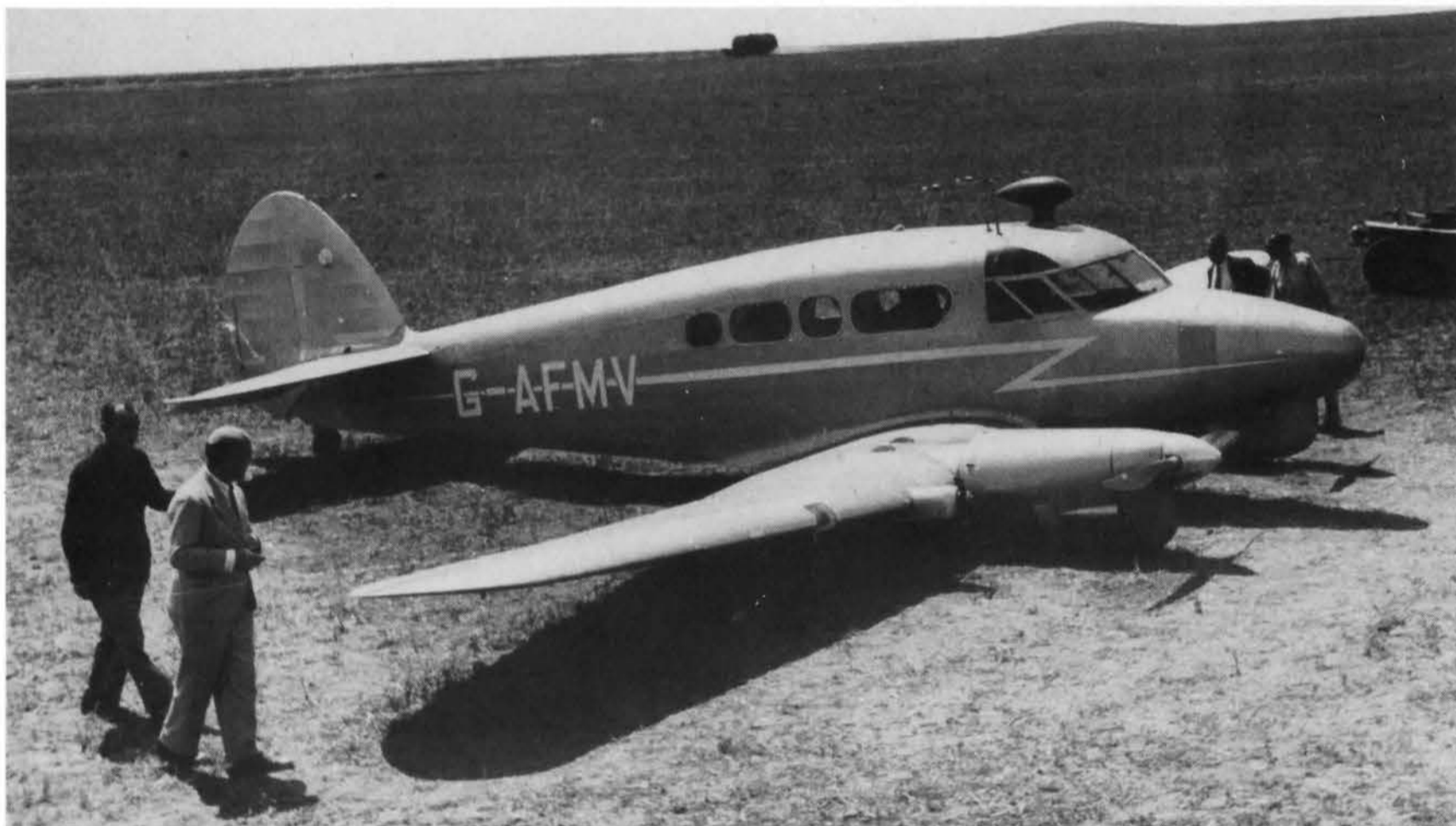
Top: Lockheed 12 EI-ALV on a visit to Gatwick in June 1963. (Peter Keating) Above: Aero Commander 680FP EI-AVP at Toussus 1.6.73. (Colin Vangen) Below: The Q6 G-AFMV after bellylanding at Constanza, Romania on 31.7.39 when the undercarriage failed. (via M.Burrow)
