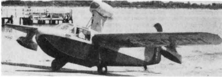
Above: "Flight" showed NC5500M with wheels retracting into the wing roots and a narrower engine support pillar with external bracing. (Both via Jack Meaden)
