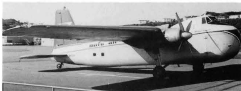
Top: Bristol Freighter ZK-CLT which was used by SAFE Air on passenger services to the Chatham Islands and therefore retained its forward fuselage windows. (R.W.Kerr)
