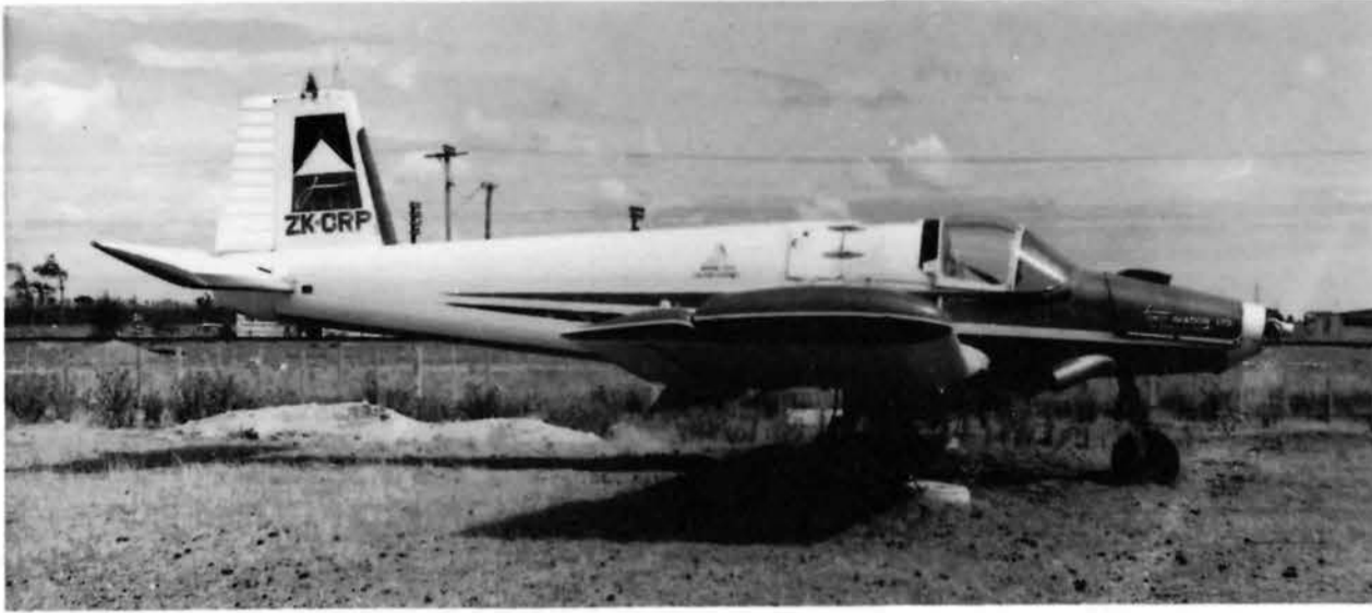
Left: Fletcher FU-24 ZK-CRP of James Aviation was one of many modified during the seventies to -950M standard, which involved replacing the six-cyl Continental engine with an eight-cyl 400hp Lycoming IO-720-A1B. (R.W.Kerr)
