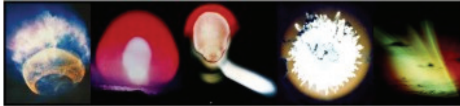
Figure 10-1. From left to right, the ORANGE, TEAK, KINGFISH, CHECKMATE, and STARFISH high-altitude nuclear tests conducted in 1958 and 1962 by the United States near Johnston Island in the mid-Pacific. Burst conditions for each were unique, and each produced strikingly different phenomena and different enhancements of the radiation belts.
