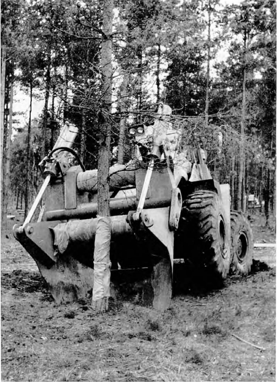
PLATE 10: A Transplanting Machine digs up an established tree complete with its root-ball.
