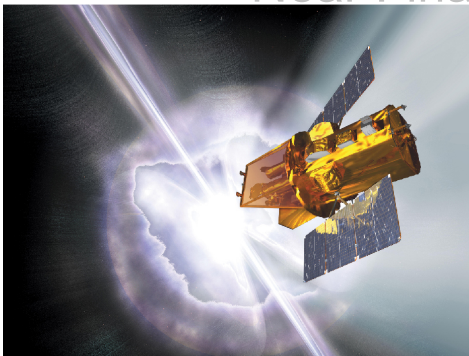
Figure 23.23. Artist's Illustration of Swift. The US/UK/Italian spacecraft Swift contains on-board gamma-ray, X-ray, and ultraviolet detectors, and has the ability to automatically reorient itself to a gamma-ray burst detected by the gamma-ray instrument. Since its launch in 2005, Swift has detected and observed over a thousand bursts, including dozens of short-duration bursts. (credit: NASA, Spectrum Astro)
