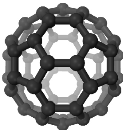
Figure 20.8. Fullerene C60. This three-dimensional perspective shows the characteristic cage-like arrangement of the 60 carbon atoms in a molecule of fullerene C60. Fullerene C60 is also known as a “buckyball,” or as its full name, buckminsterfullerene, because of its similarity to the multisided architectural domes designed by American inventor R. Buckminster Fuller.
