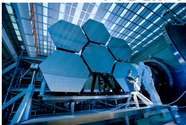
Figure 6.23. James Webb Space Telescope (JWST). This image shows some of the mirrors of the JWST as they underwent cryogenic testing. The mirrors were exposed to extreme temperatures in order to gather accurate measurements on changes in their shape as they heated and cooled. (credit: NASA/MSFC/David Higginbotham/Emmett Given)
