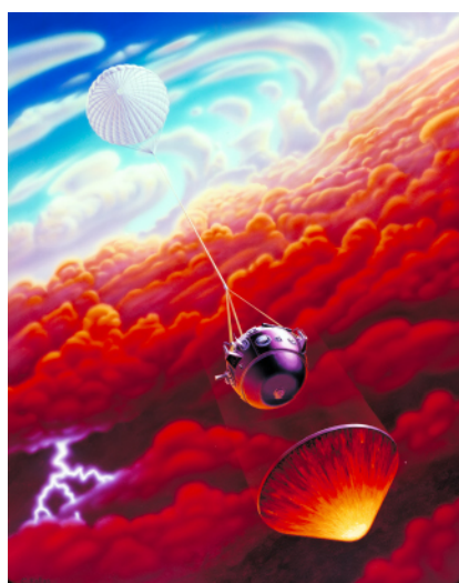
Figure 11.3. Galileo Probe Falling into Jupiter. This artist's depiction shows the Galileo probe descending into the clouds via parachute just after the protective heat shield separated. The probe made its measurements of Jupiter's atmosphere on December 7, 1995. (credit: modification of work by NASA/Ames Research Center)
