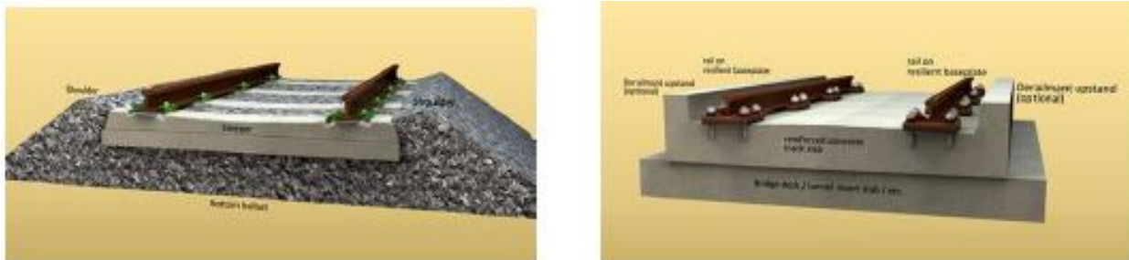
Plate 2-3. Ballasted (left) and ballast-less (right) track (Modified LRT 6 FS, 2018).
