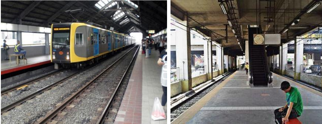
Plate 2-4. Example of side platform (left photo) and island platform (right photo) stations.
