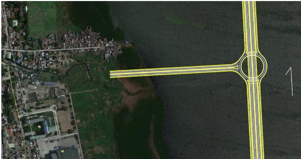
Figure 45 Proposed Grade-Separated Roundabout Interchange, Tunasan Interchange
