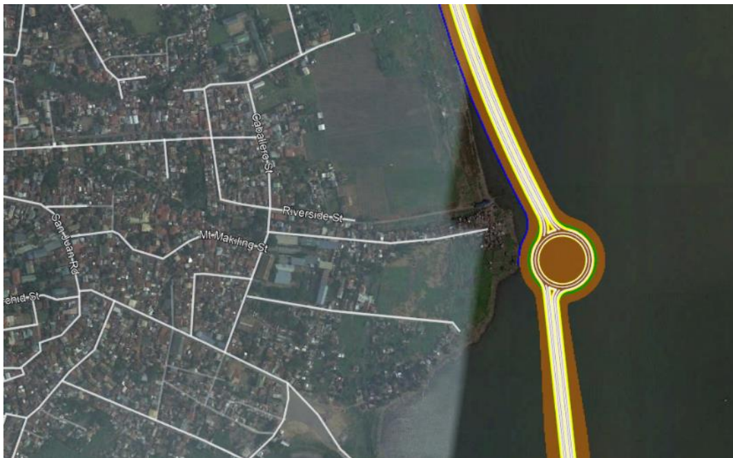
Figure 49 Current Proposed At-Grade Roundabout Interchange, Calamba Interchange
