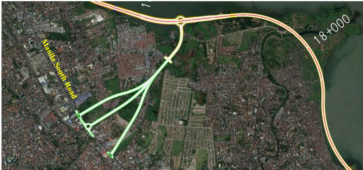
Figure 57 Proposed schemes to connect Manila South Rd for San Pedro / Binan Interchange
