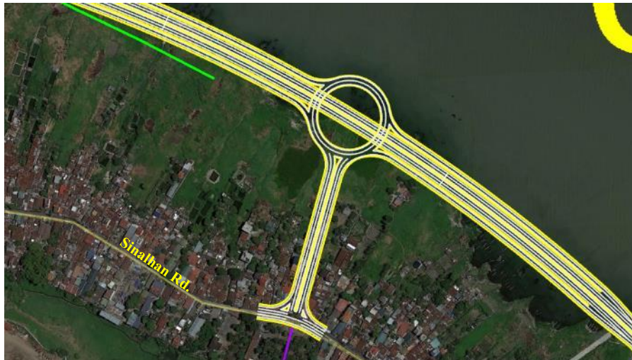
Figure 47 Proposed Grade-Separated Roundabout Interchange, Sta. Rosa Interchange
