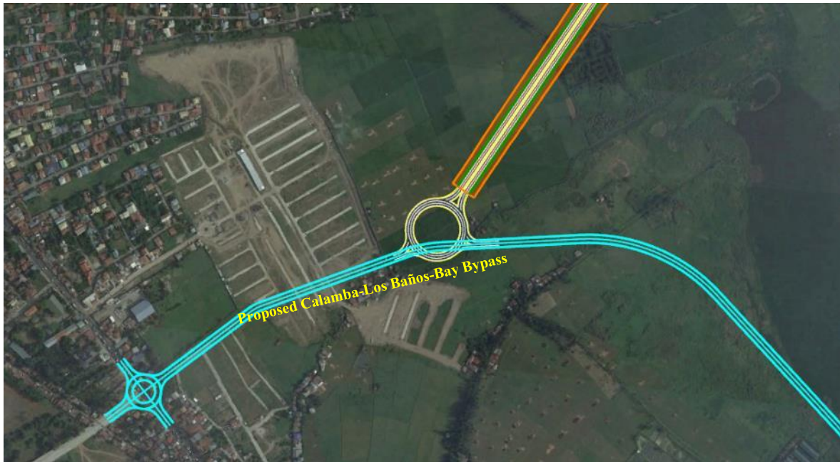
Figure 50 Proposed Roundabout Interchange with Interface Project, Calamba-Los Baños-Bay Bypass
