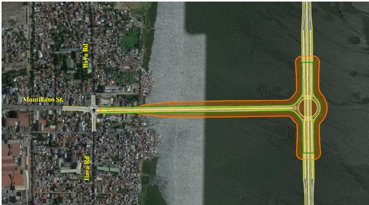
Figure 44 Proposed Grade-Separated Roundabout Interchange, Alabang Interchange
