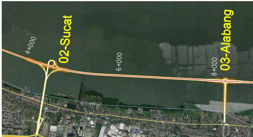
Figure 28 Sucat, Alabang Embankment required Ground Treatment
