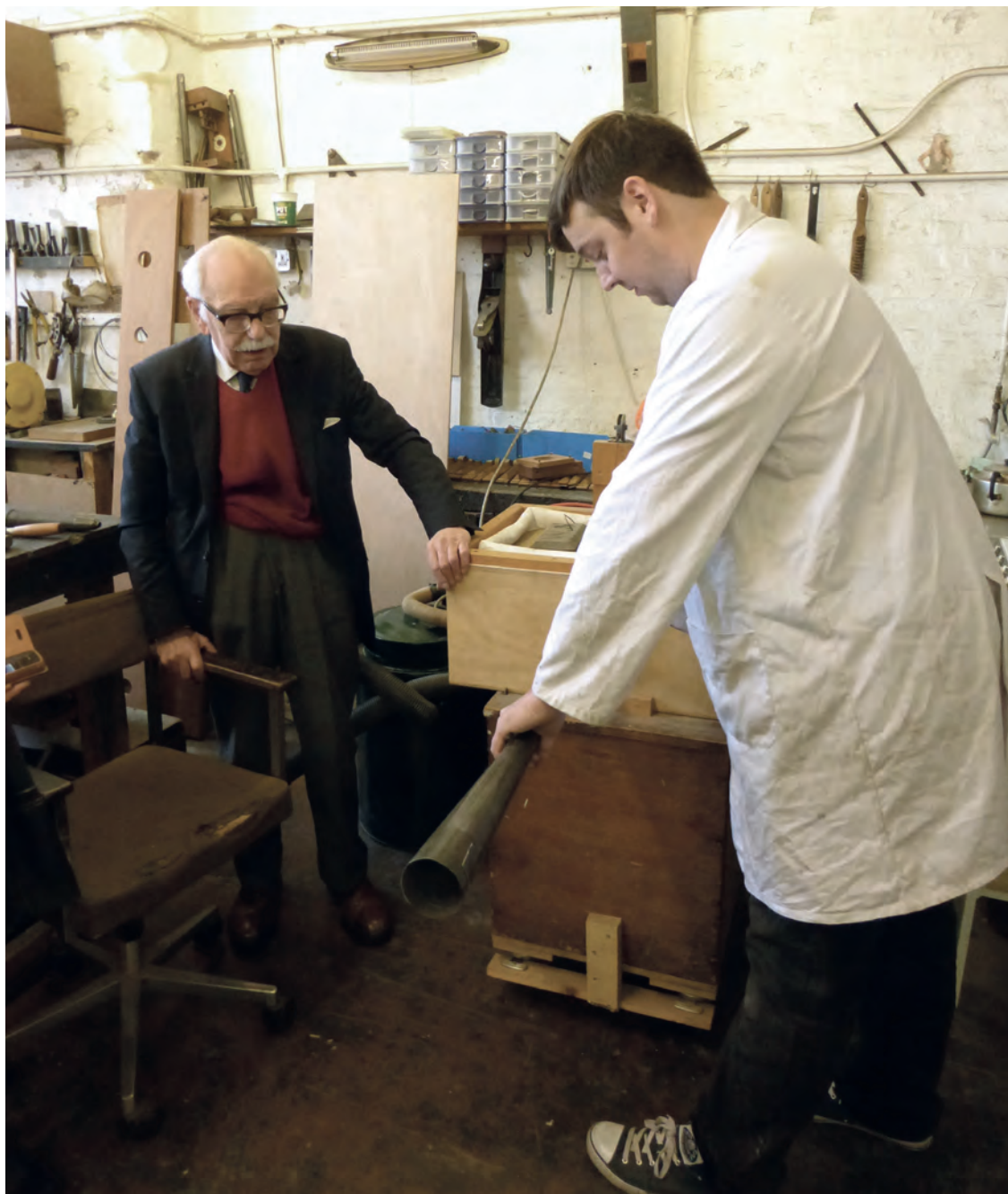
45. Organ pipe with resonator connected to a bellows machine in Maurice Merrell's workshop (Photo: Farouk Yahya)
