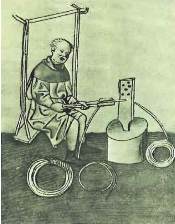
2-27. Illustration of wire drawing through a draw-plate, a manuscript of 1389 the Hausbuch , compiled in Germany by the Mendel Brothers
