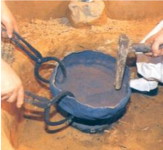
2-24b. Stretching the wall of the vessel and checking the evenness during the hammering
