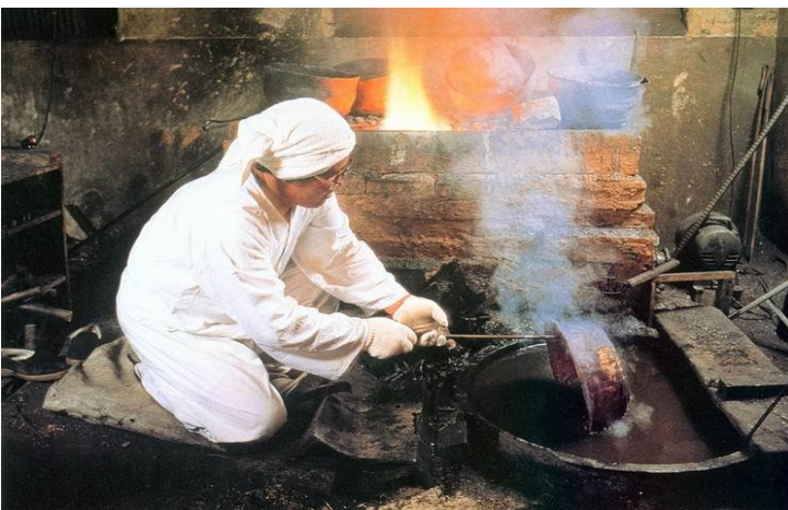
2-24c. Quenching in the yugi manufacturing process
