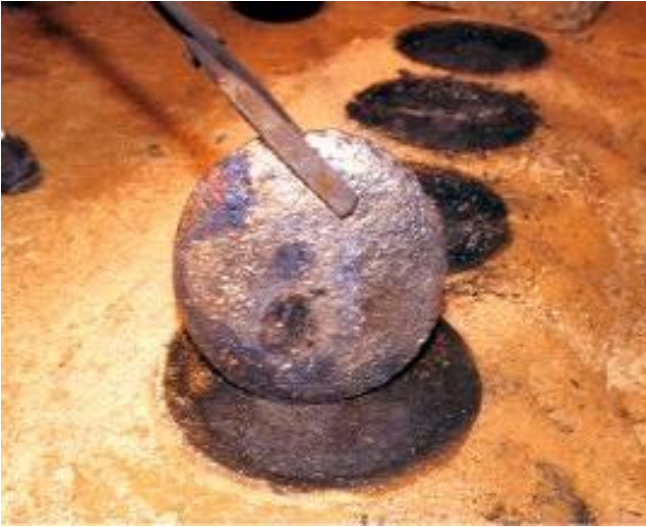
2-24a. A block of alloy moving to the anvil from the crucible
