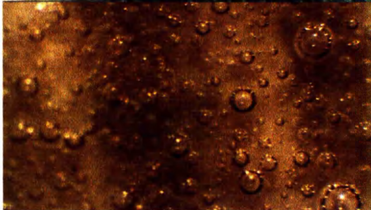
Fig. 304 Sample E: magnified glaze (40x)
