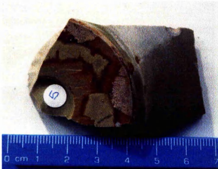
Fig. 324 Sample G: foot with marks left by spacers
