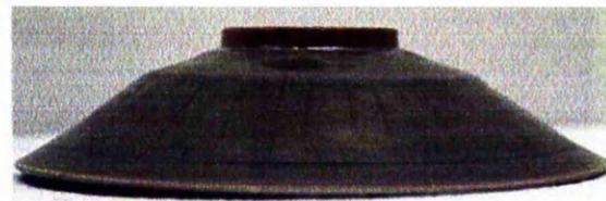
Fig. 100 Moulded pan dish showing radiating lines on the outside
