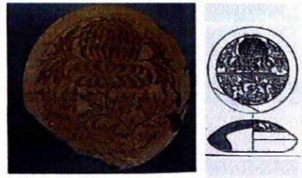
Fig. 98 Hump mould for impressing a complex design on the inner surface of a bowl
