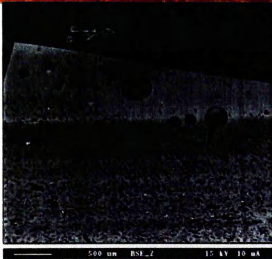
Fig. 319 Sample F: microphotograph showing body and glaze
