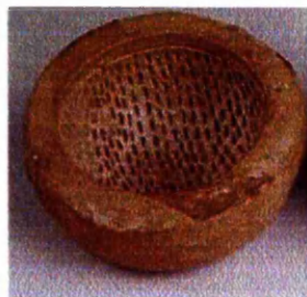
Fig. 69 One-piece outer mould with inside decoration for bei cups and cup made from similar mould
