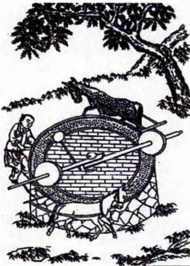
Fig. 49 Double-wheeled chaser mill pulled by two donkeys
