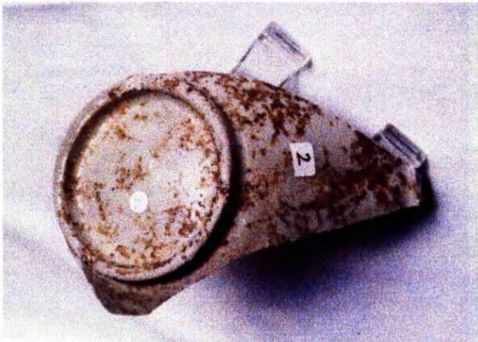
Fig. 261 Sample B: foot with gritty adhesions
