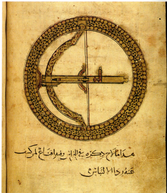
XXI Ibn Murda al-Tarsusi, al-Tabsira fi 'l-Hurub ('Manual on warfare'), Egypt or Syria, late 12th century, for the library of Saladin. Oxford, Bodleian Library, Ms. Huntington 264, f. 112v. Shielded crossbow ( atras ).
