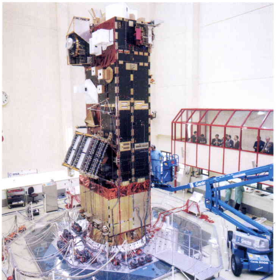
Structural model of the Polar Platform (PPF) in the Hydra Test Facility in January 1997
