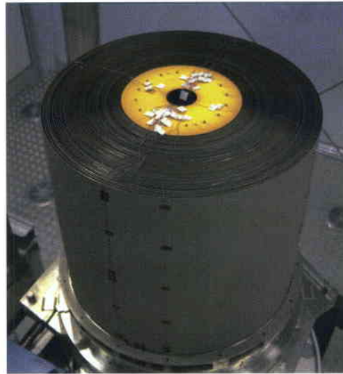
Figure 8. Mirror Module integration in progress, with 30 (left) and all 58 (right) mirrors in place.
