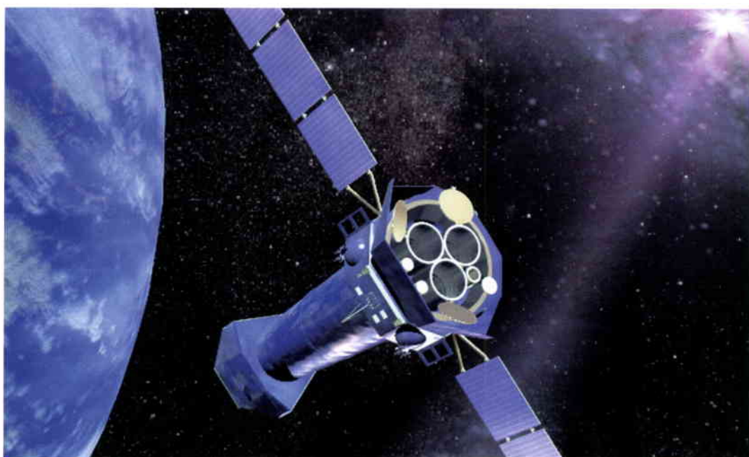
Figure 17. Artist's impression of the XMM spacecraft, with its three X-ray telescopes (courtesy of Visulab)
