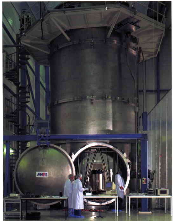
Figure 15. Focal-X facility of Centre Spatial de Liège (CSL) with the qualification-model Mirror Module inside ready for testing
