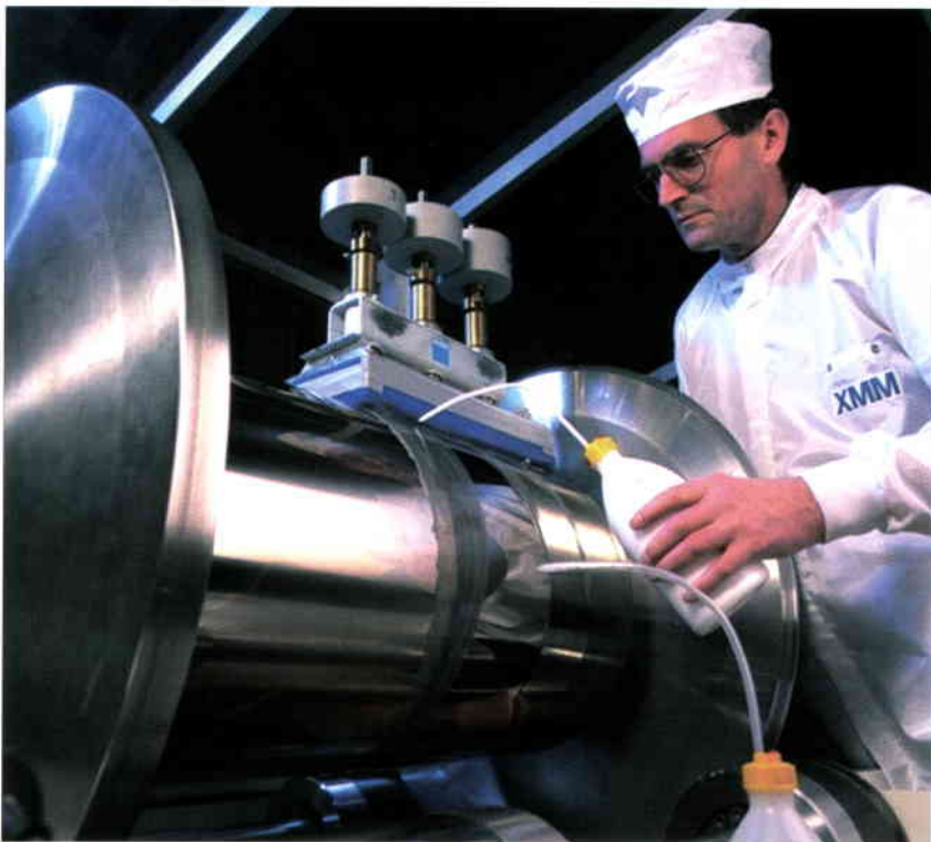
Figure 6. Mandrel super-polishing in progress
