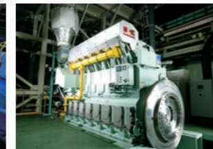
Natural gas combustion engine for shipping vessels equipped with hybrid propulsion system
