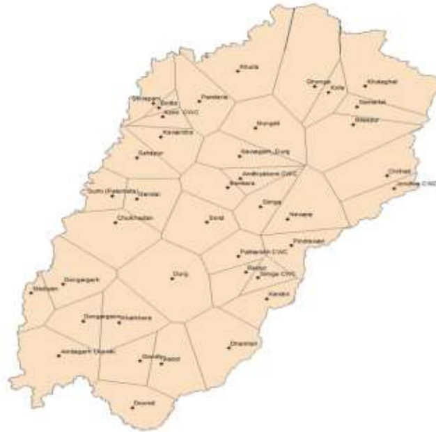
Fig. 1 – Seonath Basin with the raingauges and their corresponding Thiessen polygons
