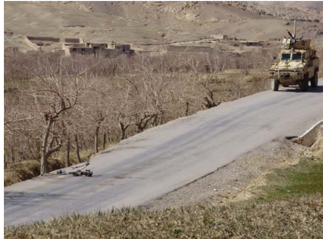
Figure A-4 A Foster-Miller robot is deployed to place a charge for a controlled detonation of an IED detected by a manned vehicle's sensor system. Note the standoff distance between the robot and the Mine Resistant, Ambush Protected (MRAP) vehicle.
