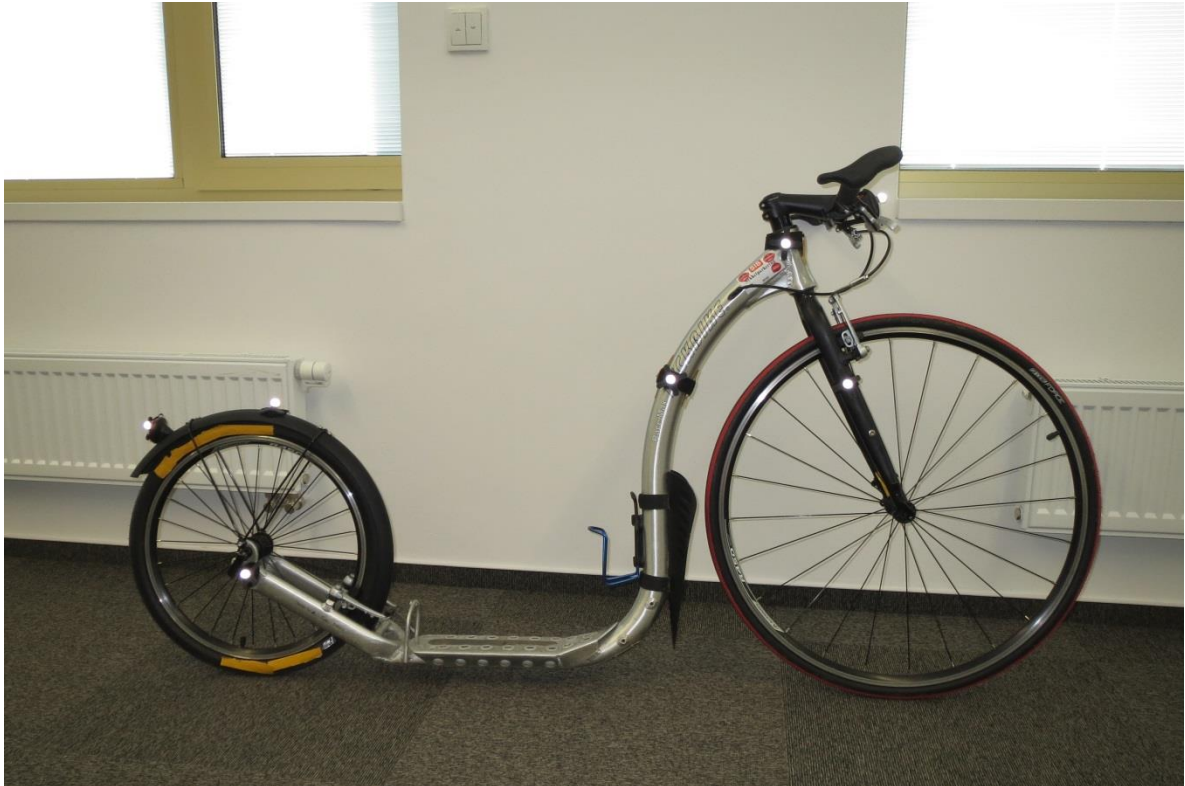
Figure 20: The Kickbike Race Max 20 scooter arranged for the kinematic recording of scooter riding. The reflexive trackers are installed and the scooter safety features are covered (author's archive).
