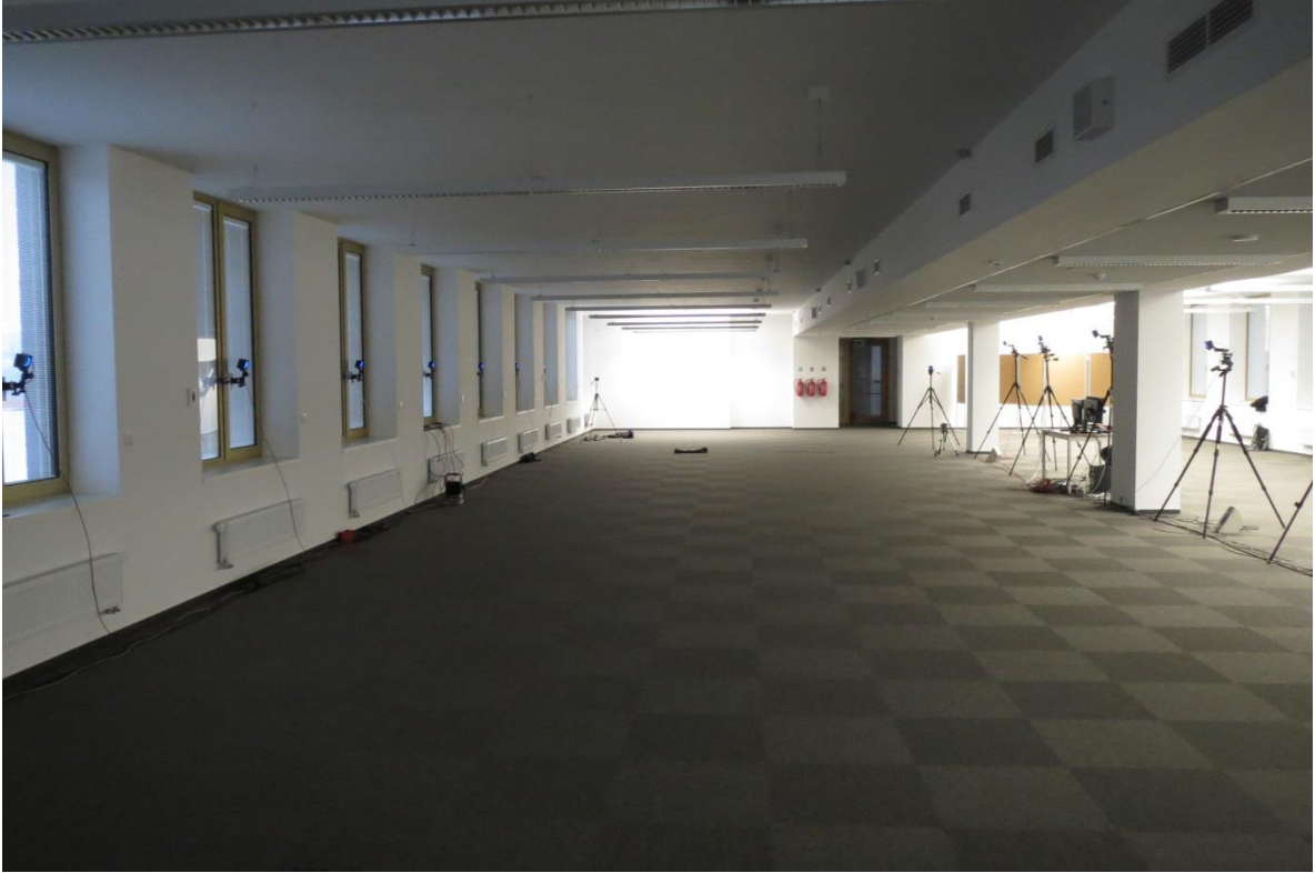
Figure 19: The monitored corridor for recording of scooter ride. There are 8 cameras installed at the windows and 8 cameras installed on the stands (author's archive).
