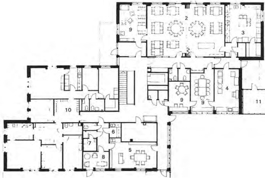
The ground floor of Prästgårdshagen. It was designed to stimulate spontaneous use of common spaces. Legend: 2. dining room; 3. kitchen; 4. laundry; 5. ceramics workshop; 6. photo lab; 7. sauna; 8. sitting/rest room; 9. club rooms/office space; 10. day-care centre for children; 11. bicycle parking.
