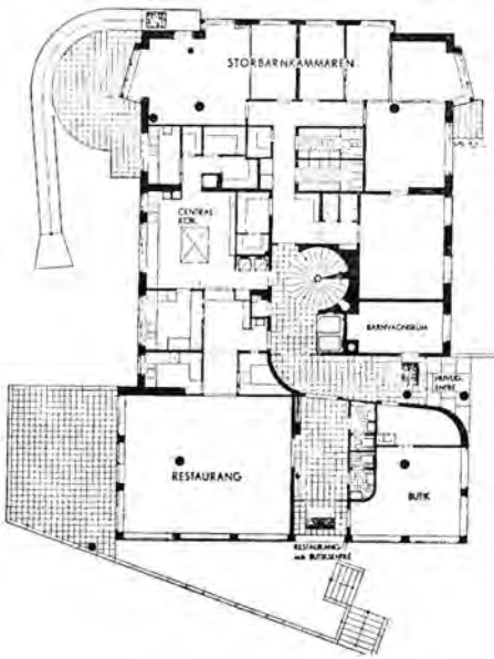
Ground floor of the YK-huset cohousing development in Stockholm, built in the 1930s. Meals were brought to the apartments through food lifts from the central kitchen. The restaurant was open to the general public.
