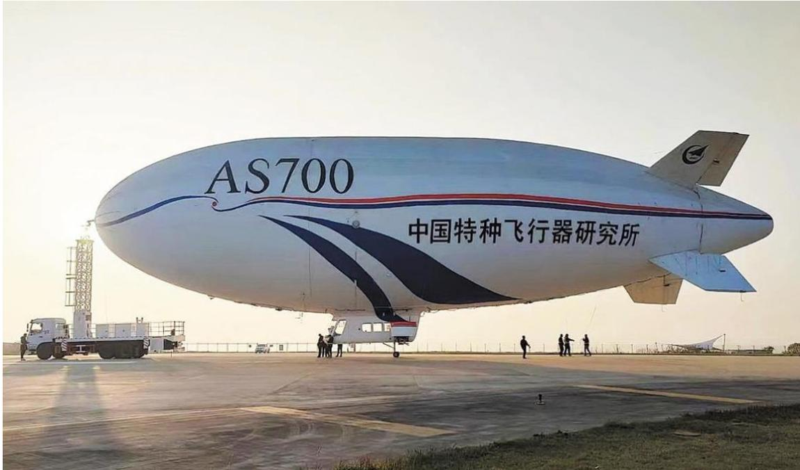
*Side view of an AS700 prototype at its mobile mooring mast.
