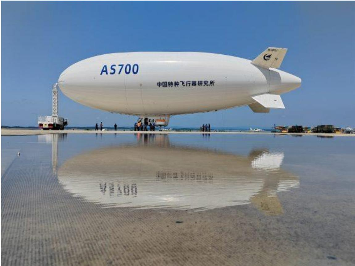
*Side view of AS700 prototype on its mobile mooring mast.
