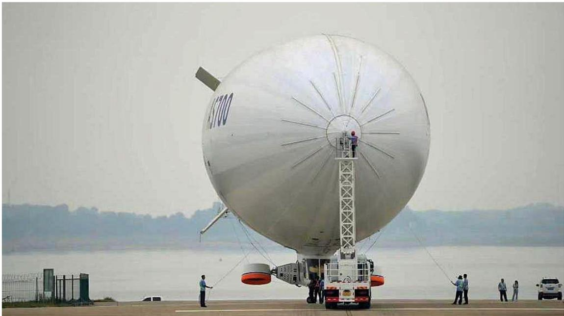
*Bow view of an AS700 prototype on its mobile mooring mast.
