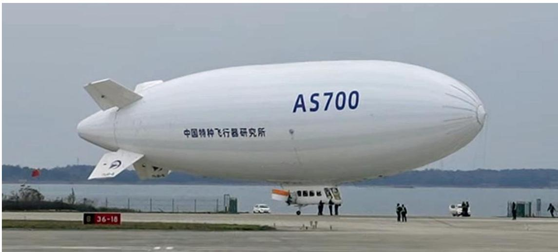
*Side view of AS-700 prototype on the ground on its single-point landing gear
