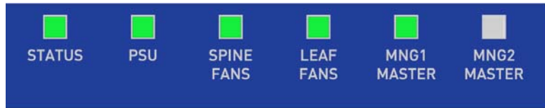
Figure 62: Spine Side Panel Display Status Indications
