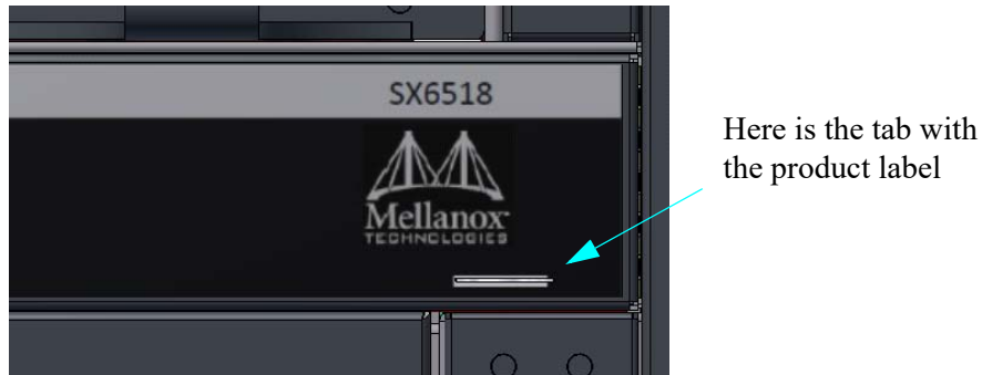
Figure 2: Product Label Tab Location
