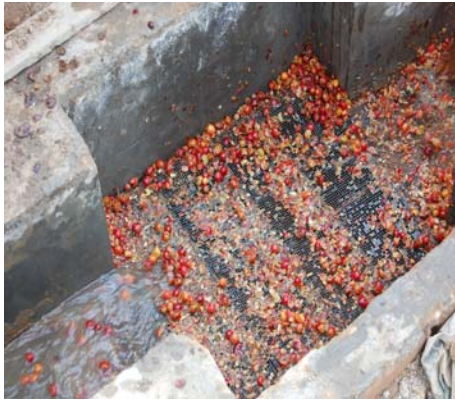
Separation of pulp from wastewater
