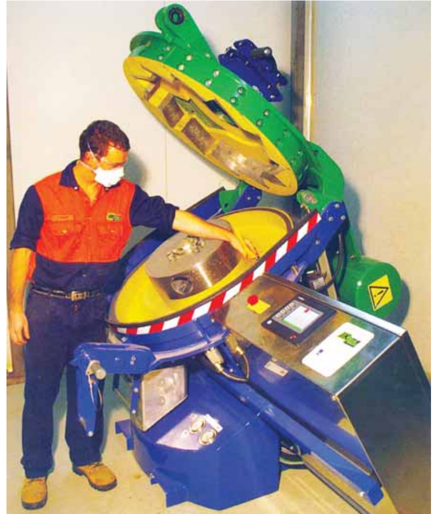
Using the rotary breakage tester on-site at the JKMRRC
