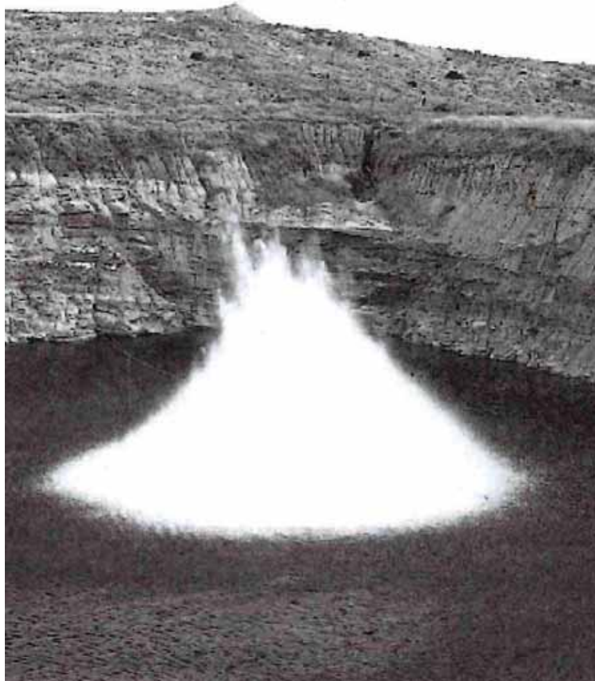
Eruption from underwater blasting test
