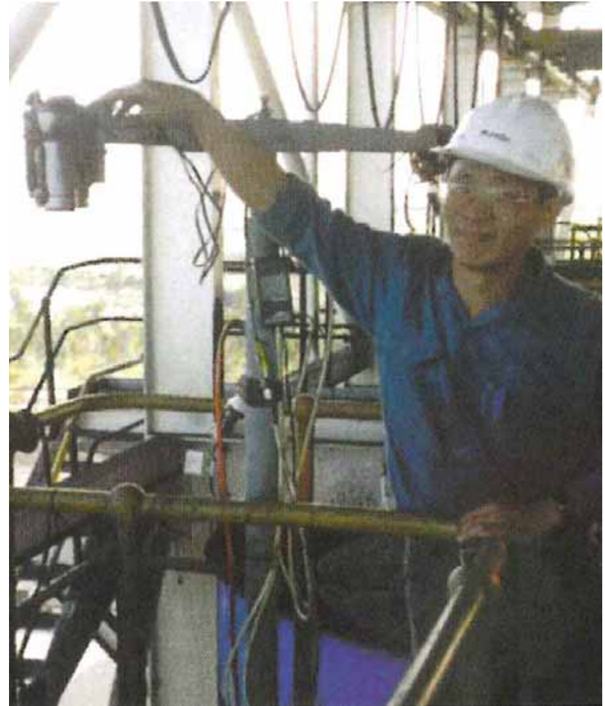
Installation of JKFrothCam
