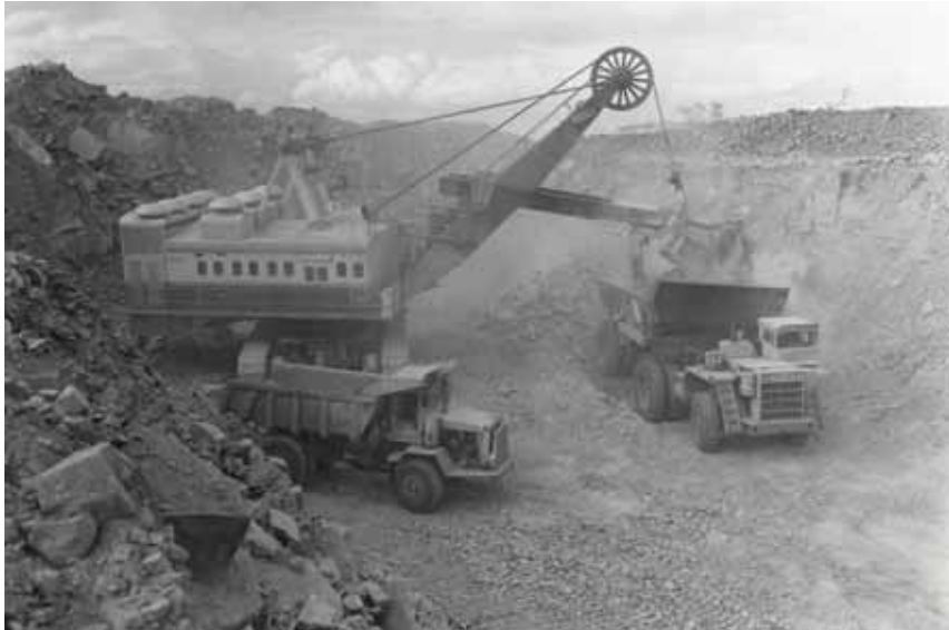
A giant power shovel operates in the Pilbara area alongside 95-tonne trucks
