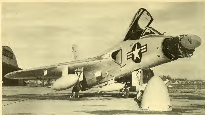
FIG. 10-10-a A Typical Transonic Radome Resting on the Concrete Apron in Front of the F4D Aircraft, Showing the Fire-Control Radar and Antenna Exposed in the Nose Section.
