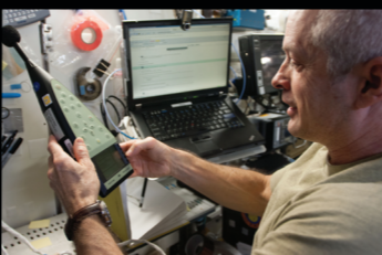
NASA astronaut Steve Swanson with Sound Level Meter (SLM) to take noise level measurements.
