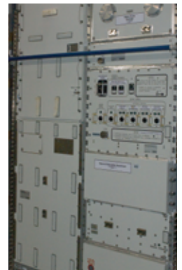
Science experiment rack accommodating a gradient furnace for material studies.
