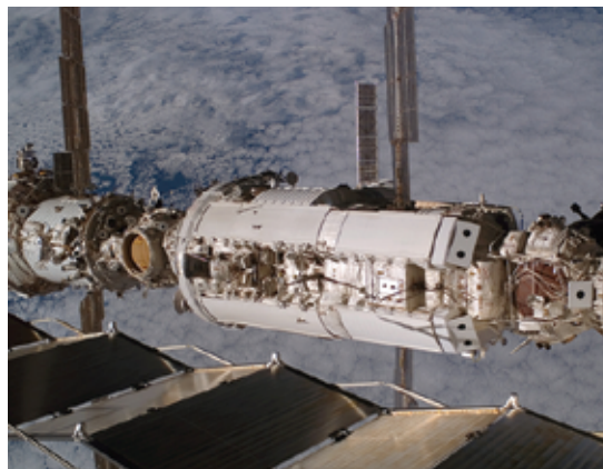
View of the FCB on orbit flanked by the Service Module and PMA-1.
