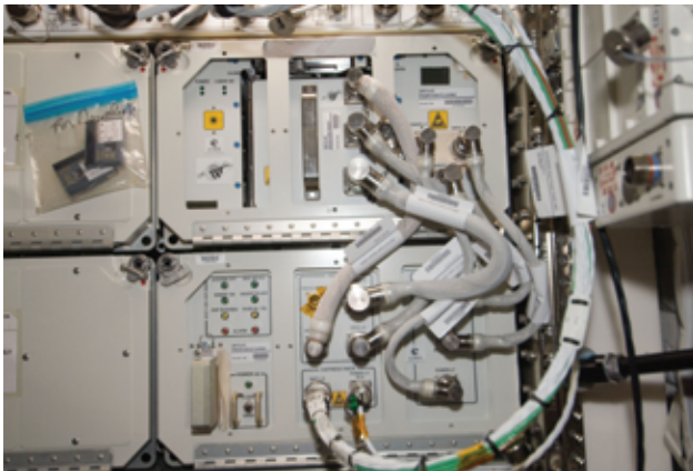
View of DDevice for the study of Critical Liquids and Crystallization (DECLIC) Experiment Locker.
