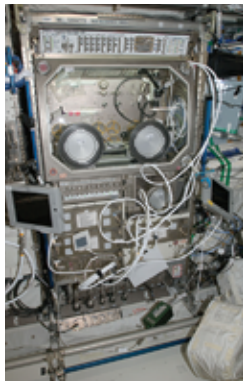
A dedicated science facility that provides a sealed environment to perform many different types of small "glovebox" sized experiments.
