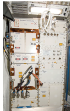
A multi-user facility for conducting fluid physics research in micro-gravity conditions.
