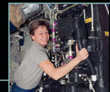
Carbon Dioxide Removal Assembly (CDRA) adsorbs carbon dioxide from crew.
