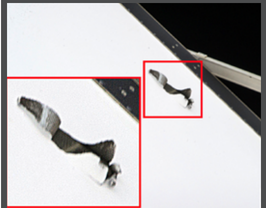
A 5 inch long by 4 inch wide hole found in 2014 in a port-side radiator for the solar array power system. No coolant leak occurred due to this impact damage.
