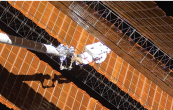
NASA astronaut Scott Parazynski, anchored to the Articulating Portable Foot Restraint (APFR) on the Orbiter Boom Sensor System (OBSS), assesses repair work on the P6 4B Solar Array Wing (SAW) as the array is deployed during an extravehicular activity (EVA).
