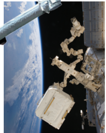
Backdropped by Earth's horizon and the blackness of space, the Canadian-built Dextre, also known as the Special Purpose Dexterous Manipulator (SPDM), is featured in this image.
