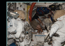
NASA Astronauts Rick Mastracchio and Mike Hopkins in the airlock (A/L). Extravehicular Mobility Units (EMUs) are visible.
