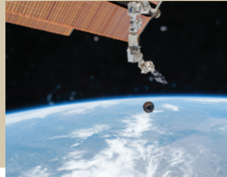
Cyclops enables the space-based launch of a new class of satellites, which are larger than cubesats but not large enough to require their own Earth-based launch vehicles.
