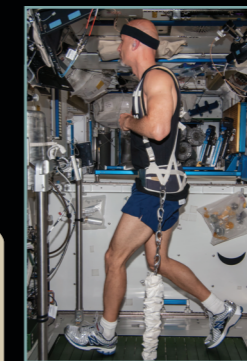
European Space Agency astronaut Luca Parmitano exercises on the Combined Operational Load Bearing External Resistance Treadmill (COLBERT).
