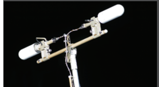
UHF antenna on the P1 Truss.
