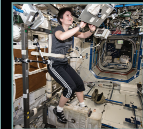
European Space Agency astronaut Samantha Cristoforetti exercises on the Cycle Ergometer with Vibration Isolation and Stabilization (CEVIS) in the Destiny Laboratory.
