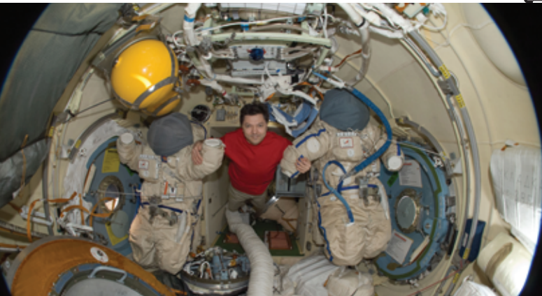
Cosmonaut Oleg Kononenko with two Russian Orlan spacesuits in the Pirs Docking Compartment.
