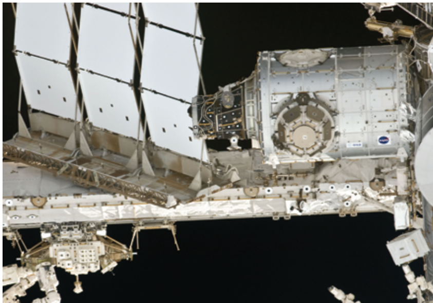
Exterior view the P1 truss segment, and the Node 3/Tranquility and Cupola.
