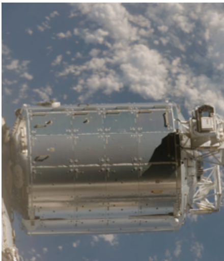
The European Columbus Research Laboratory has four exterior mounting platforms that can accommodate external payloads.
