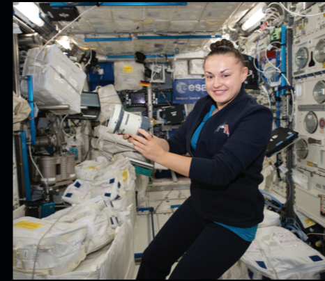
Russian cosmonaut Lena Serova RS 41FE with Microbial Air Sampler (MAS) for the Microbial Sampling investigation.
