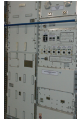
Science experiment rack accommodating a gradient heating furnace for material studies.
