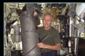
Elektron produces oxygen from water through electrolysis; vents hydrogen out of the station.
