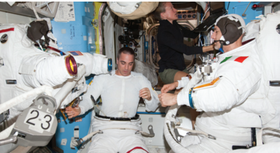
View of NASA astronaut Chris Cassidy (left) and European Space Agency astronaut Luca Parmitano (right) preparing for a dry run in the International Space Station's Quest airlock in preparation for the first of two sessions of extravehicular (EVA). Both are wearing a liquid cooling and ventilation garment and preparing to don their EMUs. Astronaut Karen Nyberg, is visible in the foreground.
