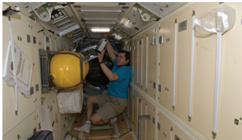
Russian cosmonaut Oleg Skripochka uses the Russian Tekh-38 VETEROK ("Breeze") science hardware to take aero-ionic concentration measurements in the Rassvet Mini-Research Module 1 (MRM1).
