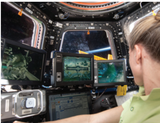
At the robotics workstation in the Cupola, NASA astronaut Karen Nyberg participates in onboard training activity in preparation for the grapple and berthing of a visiting vehicle.
