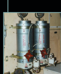
Solid Fuel Oxygen Generator (SFOG), burns candles to produce oxygen as a backup system.
