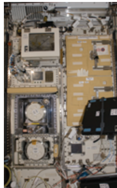
A multipurpose payload rack system that sustains life science experiment units inside and supplies resources to them.
