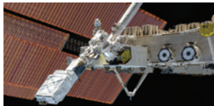
Small Satellite Orbital Deployer (SSOD) providing a novel, safe, small satellite launching capability.
