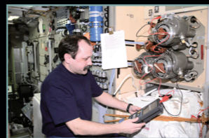
Vozdukh absorbs carbon dioxide from crew.
