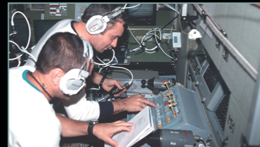
Crew uses Progress Remote Control workstation in SM.
