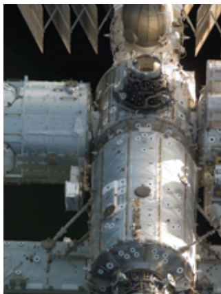
Visible are the Pressurized Mating Adapter 2 (PMA2), Destiny laboratory module, and Node 1.
