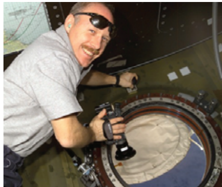
U.S. Lab in orbit, above, NASA astronaut Ken Bowersox uses camera at window with partially deployed shutter; to right, window shutter fully deployed; outer debris shields are visible.
