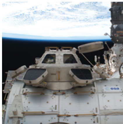
Exterior view of the Cupola and the Node 3/Tranquility taken by a crew member during a Extravehicular Activity (EVA). Crew members onboard are partially visible in the Cupola windows.
