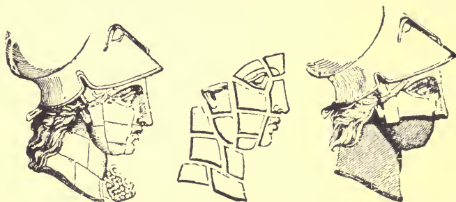
FIGS. 78, 79, 80.—SHOWING THE SUPPOSED METHOD OF WORKING IVORY IN PIECES LAID ON.
