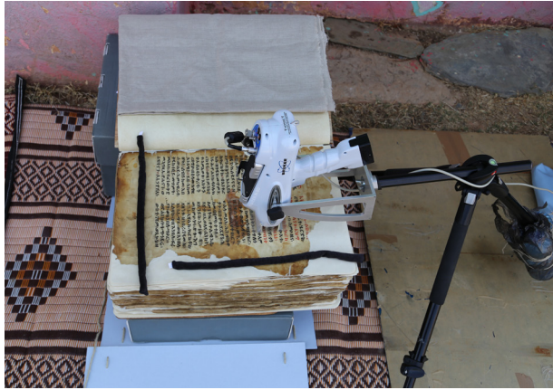
Fig. 5. 'Ura Qirqos, June 2014: examining the inks with the help of X-ray fluorescence spectroscopy.
