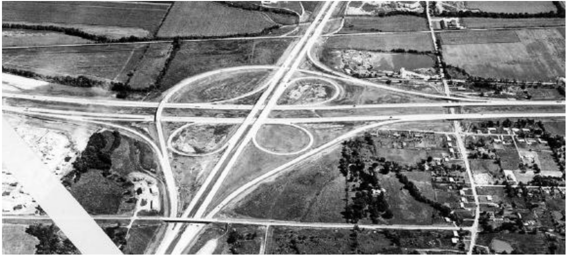
Exhibit 10-40. Four-Leg Interchange, Cloverleaf With a Semidirect Connection
