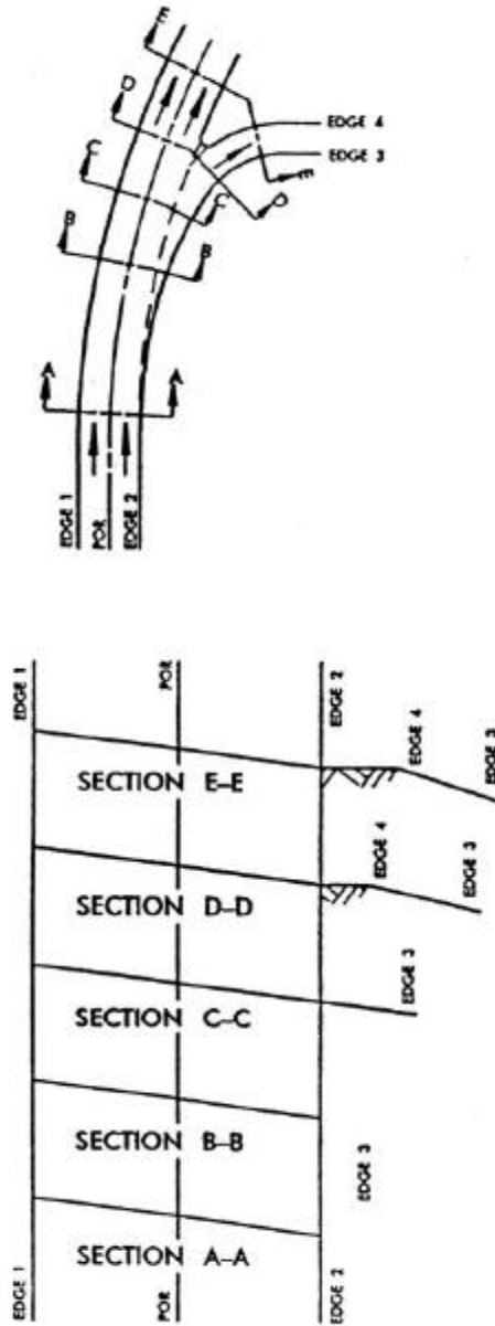
Exhibit 9-46. Development of Superelevation at Turning Roadway Terminals
