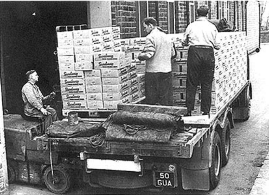
Above: Cases of soft-drinks cans stacked on to a lorry by hand from a fork-lift truck in the early 1960s.
