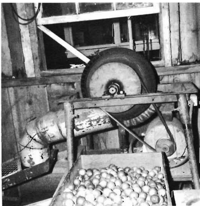
Figure 87. Rubber-tire husker with its power source an electric motor, still used by Francis Takahashi on Kauai.
