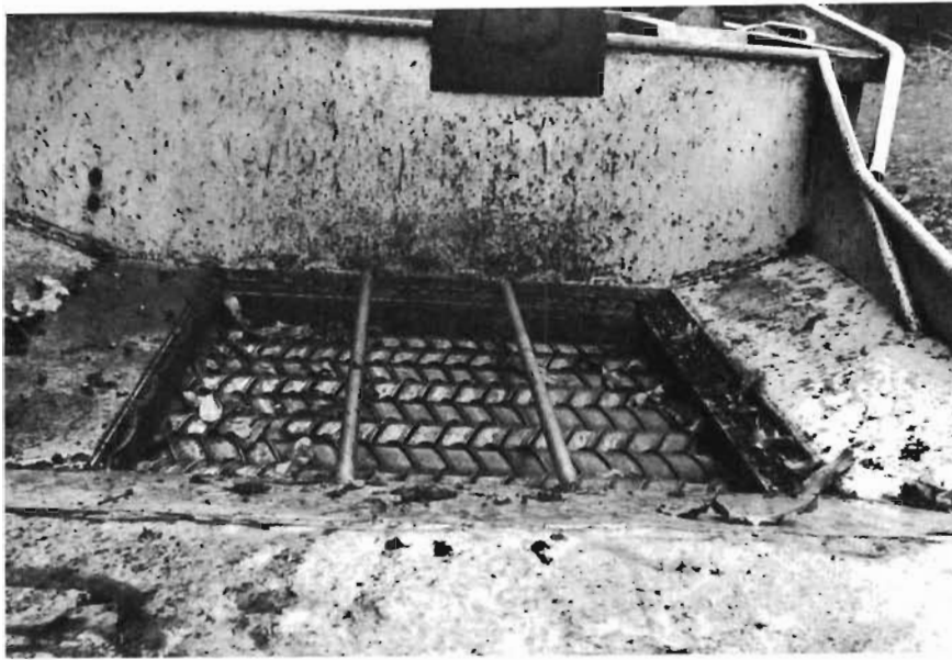
Figure 84. Leaf stripper showing the counter-rotating scrolls to separate the nuts from the leaves.
