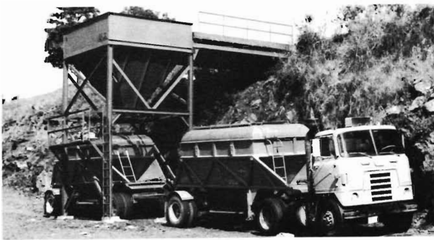
Figure 85. Bulk trailers for hauling nuts.
