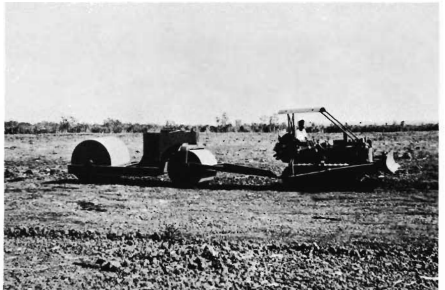
Figure 109. Land rolling at Keaau Orchard with a reclaimed steamroller, 1950. Note decided improvement in land surface. (Courtesy of Mauna Loa Macadamia Nut Corp.)
