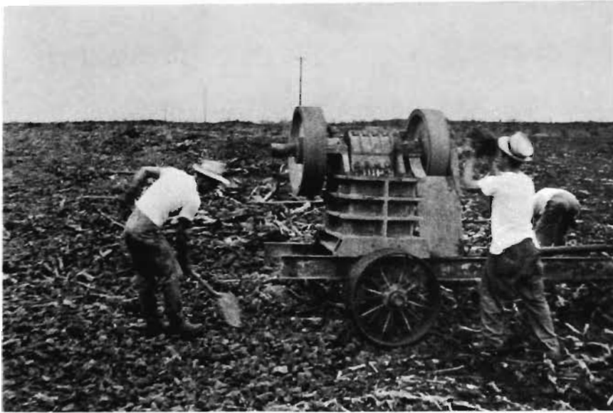
Figure 108. A test to crush large pieces of lava rock to create filler materials that would aid in water and nutrient retention in macadamia orchards, 1953. The experiment proved too costly at Keaau. (Courtesy of Mauna Loa Macadamia Nut Corp.)
