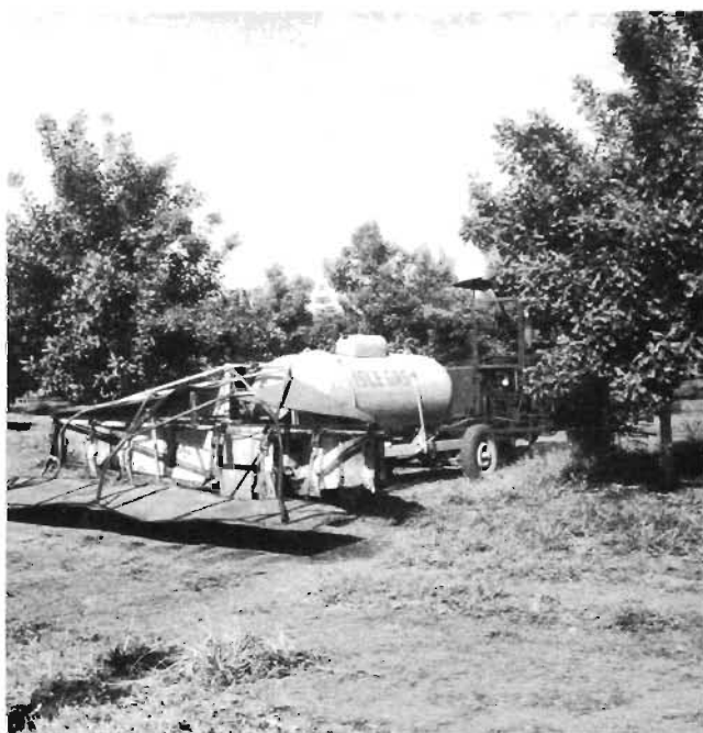
Figure 71. Flamethrower experimentally used at Keaau Orchard in the early 1960s.
