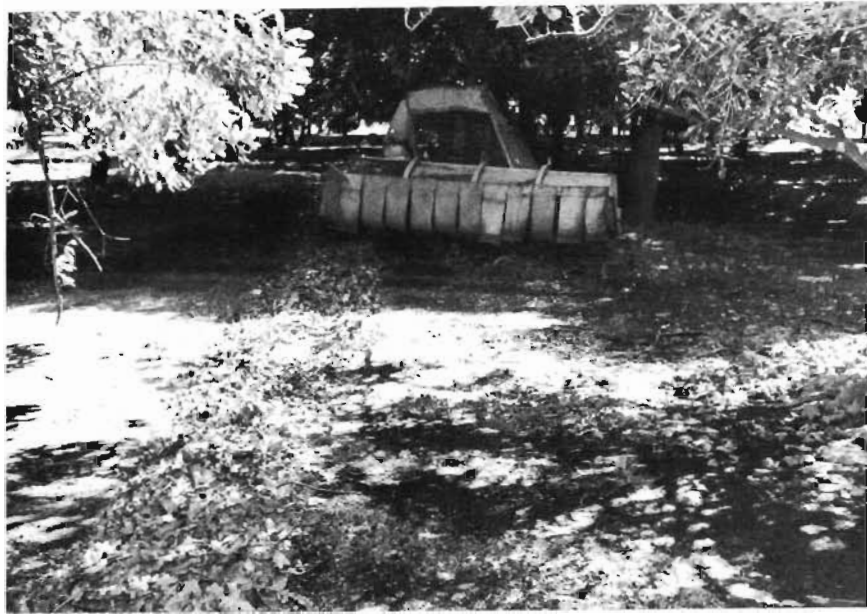
Figure 79. Sweeper used to windrow nuts in the center of the tree rows for mechanical pickup.
