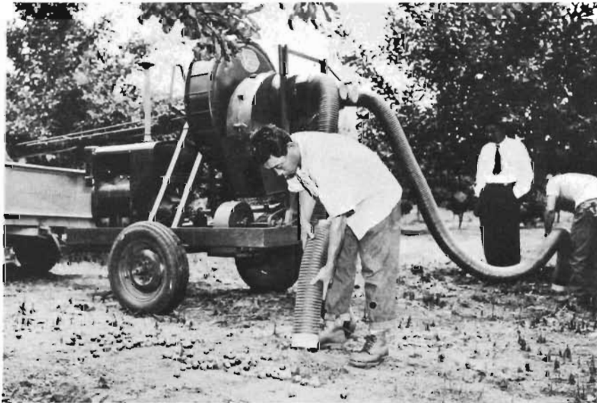
Figure 125. Experimental vacuum harvesting of macadamia nuts placed on ground at Keaau Orchard, 1953. Note quarry waste spread on ground to fill crevices. (Courtesy of Mauna Loa Macadamia Nut Corp.)
