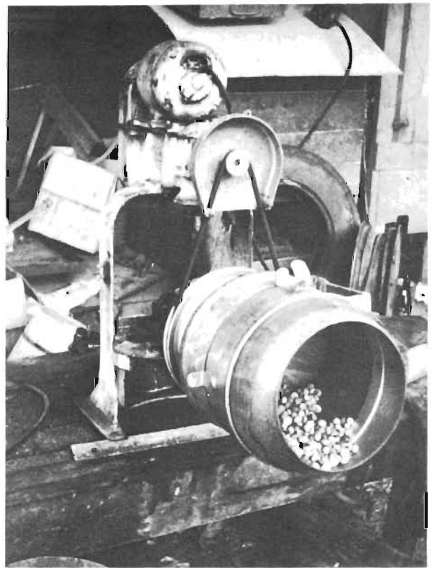
Figure 130. Separation of kernels from shells was accomplished in a rotating drum by having the shells, which are lighter in weight than the kernels, spill over the edge. The remaining shells were hand separated. The smaller pieces and fines were separated through screened portholes in the lower portion of the drum. This machine was used by Mamoru Takitani of Hawaiian Host Candy in his original candy factory in the attic of his father's soda-water-bottling building in Wailuku, Maui, about 1955.
