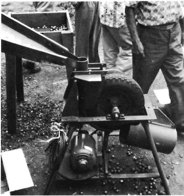
Figure 126. Made by a grower in the Kohala area, this portable nut husker uses a small wheelbarrow tire.
