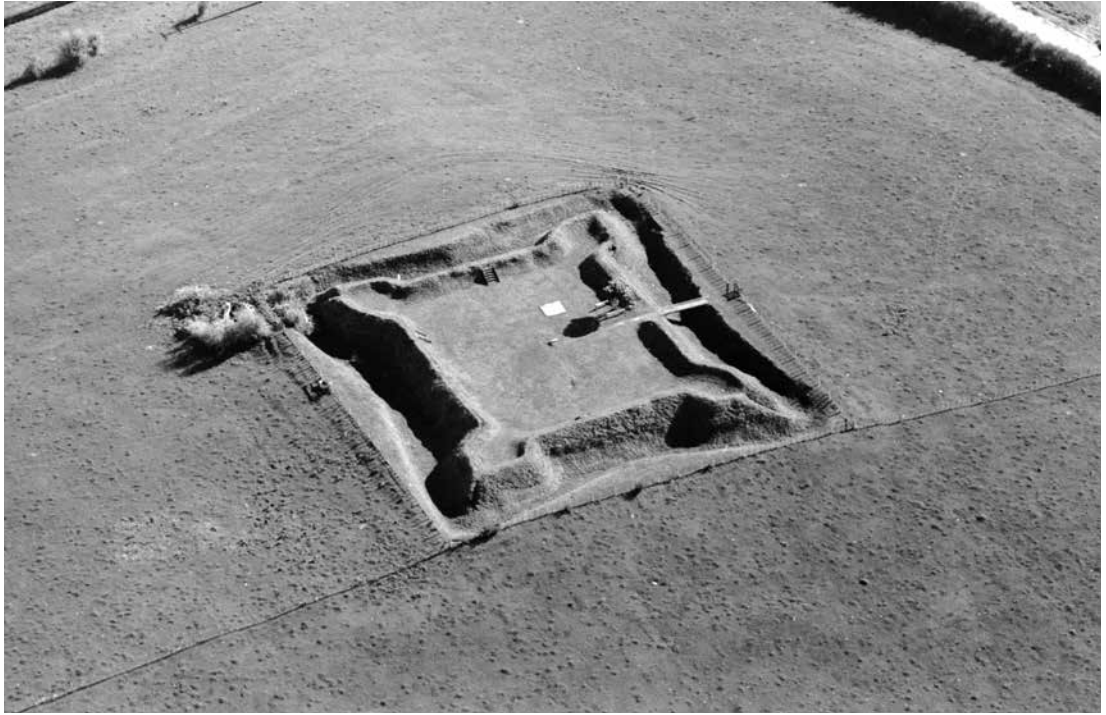
Figure 36. Alexandra Redoubt, Pirongia: bastions at four corners cover each side from both adjacent angles. Photo: Kees Sprengers, Waikato Museum Te Whare Taonga o Waikato, Ref. No M542-26 (1980).
