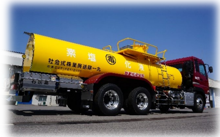
Liquid Chlorine Tank Truck
