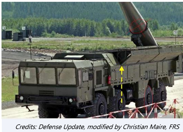
Figure 16. Relation between the diameter of the wheel of the MZTK 7930 launcher and the 9M720 SS-26E missile
