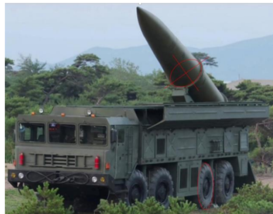
Figure 17. Relation between the diameter of the wheel of the MZTK 7930 type launcher and the KN-23 missile
