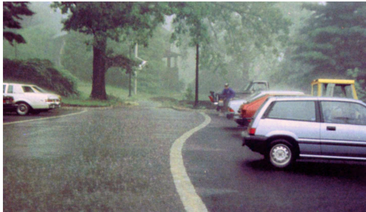
Porous paving in parking lots increases infiltration and reduces runoff
