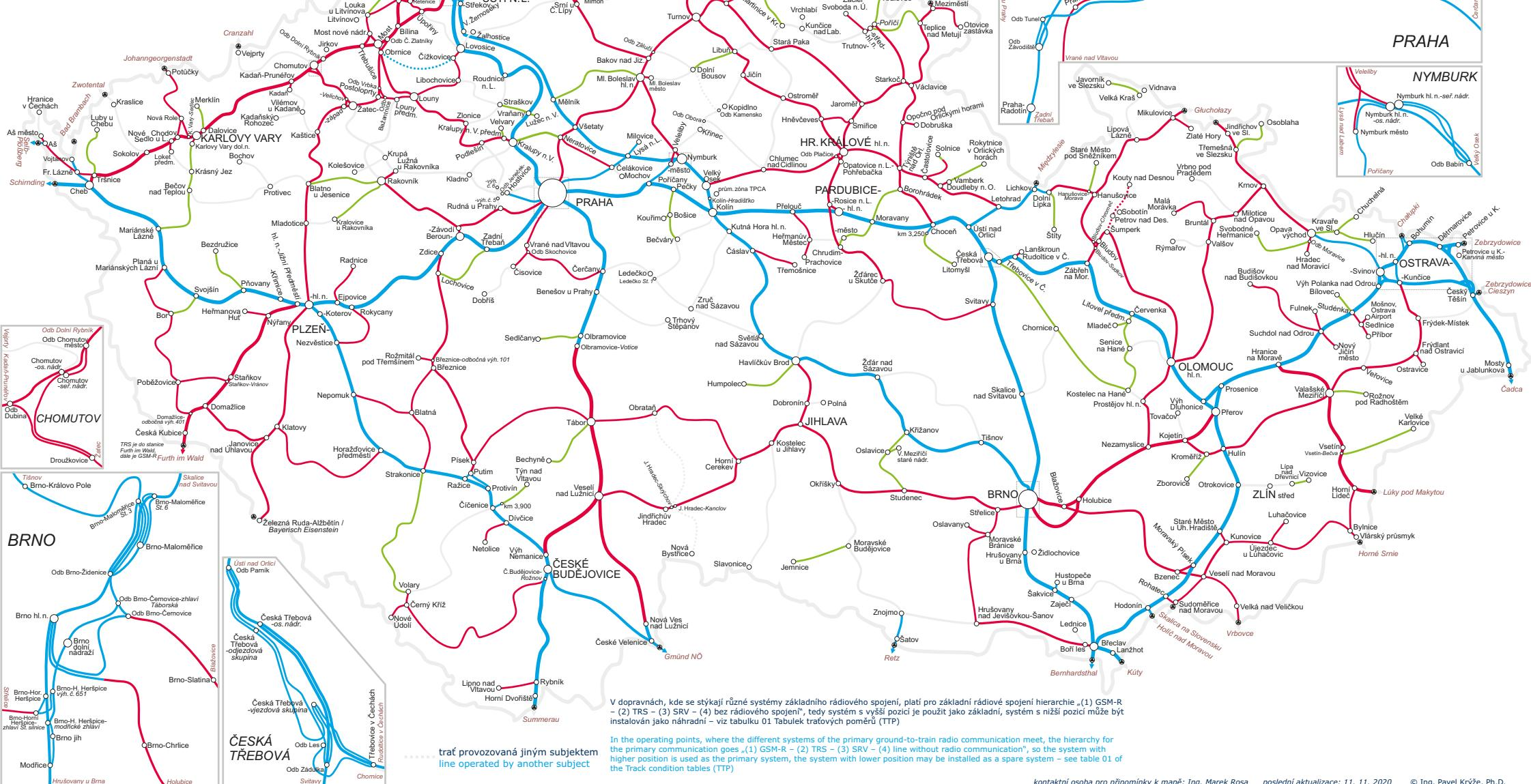
In the operating points, where the different systems of the primary ground-to-train radio communication meet, the hierarchy for the primary communication goes „(1) GSM-R – (2) TRS – (3) SRV – (4) line without radio communication“, so the system with higher position is used as the primary system, the system with lower position may be installed as a spare system – see table 01 of the Track condition tables (TPP)
