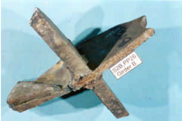
Figure 59: Web Crack Removed From Girder B at P.P. 26 at the Shelf Plate Connection
