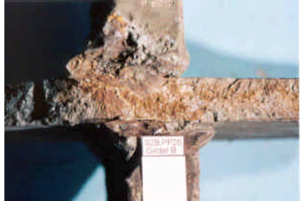
Figure 59: Web Crack Removed From Girder B at P.P. 26 at the Shelf Plate Connection
