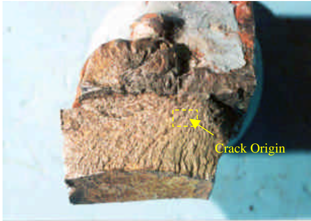
Figure 50: Opposing Crack Surfaces Showing the Web Fracture Origin Near the Weld Root (Girder E P.P. 28) (Enlarged View of Boxed Area Shown Below)
