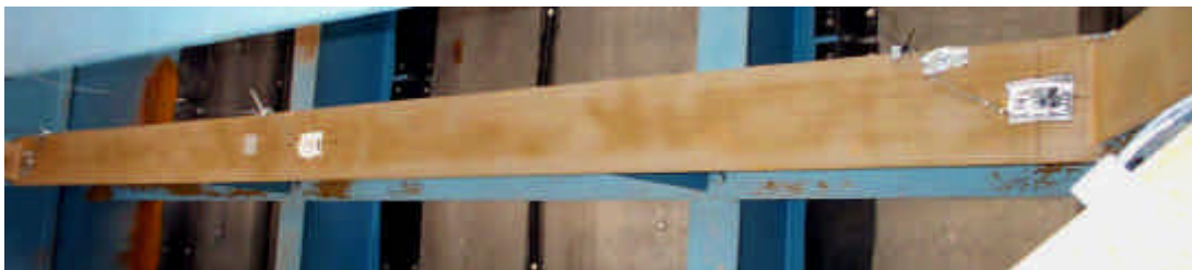
Figure 43: Photo's of Strain Gage Installation
